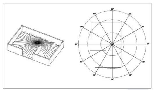
The product is mainly suitable for the navigation and obstacle avoidance of robots (e.g. floor mopping robots and service robots) by performing a 360° scan of the indoor layout and building a map so that a walking path can be planned. It is also suitable for robotics education and research, etc.
