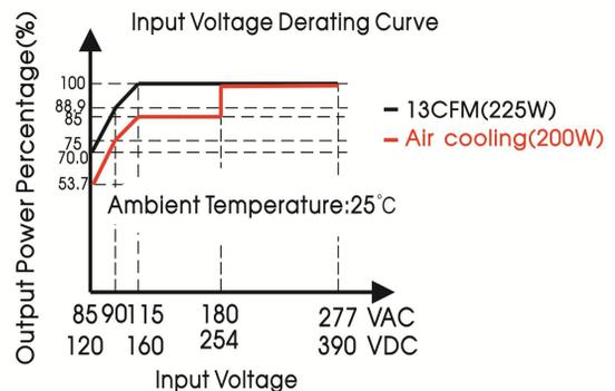
Note: 1. With an AC input voltage between 85-277VAC and a DC input between 120-390VDC the output power must be derated as per the temperature derating curves.
