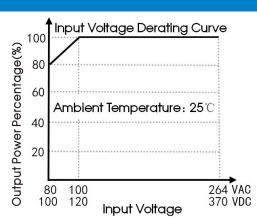
Note: ① With an AC input between 80-100VAC and a DC input between 100-120VDC, the output power must be derated as per temperature derating curves; ② This product is suitable for applications using natural air cooling; for applications in closed environment please consult factory or one of our FAE.
