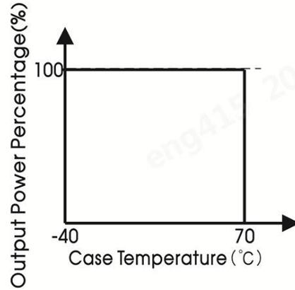
Note: 1. With an AC input voltage between 85 -180VAC and a DC input between 120 - 254VDC the output power must be derated as per the temperature derating curves;
