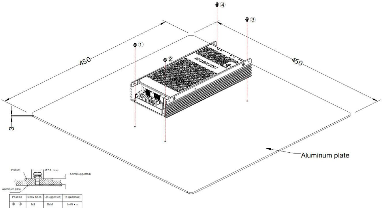
**Note:** 1. In order to meet the "Derating Curve", the product testing must be installed onto an aluminum plate. The size of the suggested aluminum plate is shown as above. And for optimizing thermal performance, it is necessary to apply thermal grease on the bottom of the product.
