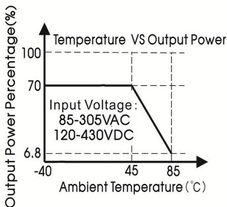
With aluminum plate for heat dissipation or 23.5CFM
