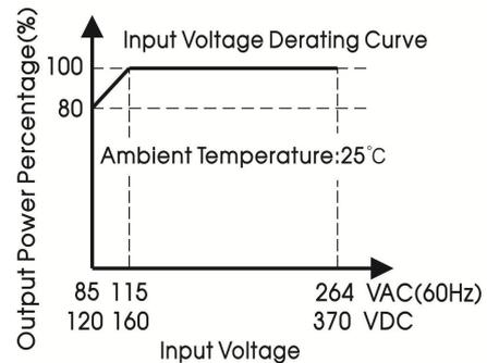
Note: 1. With an AC input voltage between 85 -115VAC and a DC input between 120-160VDC the output power must be derated as per the temperature derating curves;
