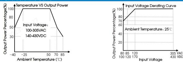
Note: 1) With an AC input between 80-120VAC and a DC input between 100-170VDC, in addition to the voltage drop, temperature derating is also required. If it is used in a low temperature environment, please consult Mornsun FAE.
