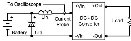
**Peak-to-Peak Output Noise Measurement Test**
