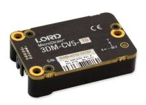
The LORD Sensing 3DM-CV5 family of industrial-grade, board-level inertial sensors provides a wide range of triaxial inertial measurements, computed attitude, and navigation solutions.
