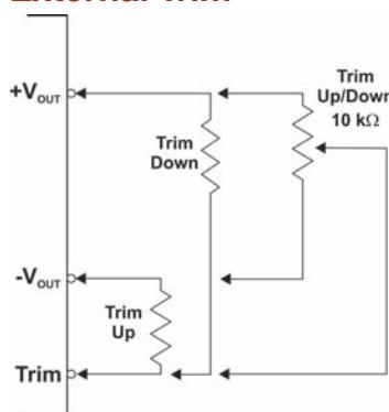
A simple external circuit may be used to adjust the converter output. To adjust the output DOWN, connect a 5%, 3W resistor between the plus output pin and the Vout trim pin. To adjust the output UP, connect a 5%, 3W resistor between the minus output pin and the Vout trim pin. To calculate the correct resistor value use:
