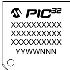
64-Lead TQFP (10x10x1 mm)
