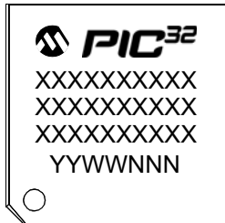
64-Lead TQFP (10x10x1 mm)
