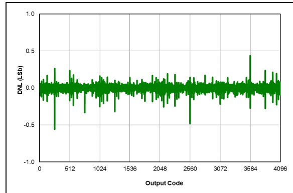
FIGURE 45-90: ADC 12-Bit Mode, Single-Ended, Typical DNL, VDD = 3.0V, VREF = 3.0V, TAD = 0.5 µs, 25°C, All devices.
