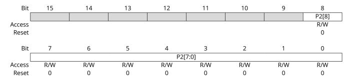
**Bit 8 – P2[8]** Parameter 2 Most Significant bit UART mode operating parameter values
