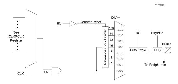
Figure 25-2. Clock Reference Timing
