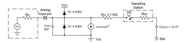
Legend: CPIN = Input Capacitance ILEAKAGE = Leakage Current at the pin due to various junctions Rıc = Interconnect Resistance Sampling Rs = Source Impedance Switch Rss  $V_A$ = Analog Voltage  $(K\Omega)$ Vт = Diode Forward Voltage SS = Sampling Switch = Resistance of the Sampling Switch Rss = Sample/Hold Capacitance 2 3 4 5 6 Vnn Note: (V)
