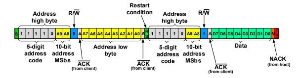
Figure 36-26. 7-Bit Host Write Diagram
