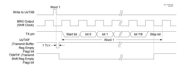
Figure 34-4. UART Asynchronous Transmission (Back-to-Back)
