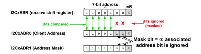
In 10-bit Address mode, I2CxADR0 and I2CxADR1, and I2CxADR2 and I2CxADR3, are combined to create two 10-bit addresses. I2CxADR0 and I2CxADR2 hold the lower eight bits of the address, while I2CxADR1 and I2CxADR3 hold the upper two bits of the address, the  $R/\overline{W}$  bit, and the five-digit '11110' code assigned to the five Most Significant bits of the high address byte.
