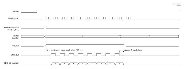
Notes: 1. SDO bit number illustrates the transmitted bit number and is not intended to imply SDO\_out tristate operation.
