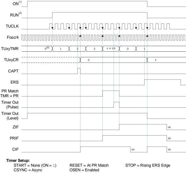
Figure 29-5. Synchronization and Prescaler Timing (CSYNC = 0)
