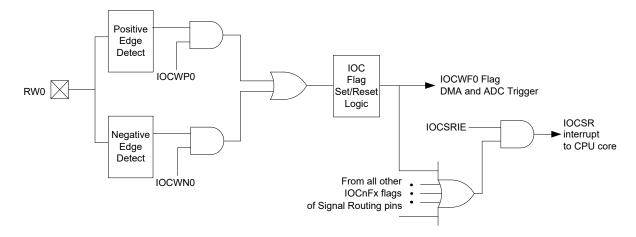
In addition to the Interrupt-on-Change, the output of each pin of the Signal Routing Port is also a trigger for the DMA and ADC as shown in the Figure 20-1. The IOCWP and IOCWN registers are used to select the edge of the output pin transition that generates a trigger.
