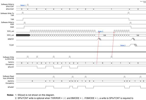
Figure 35-3. SPI Host Operation - Data Exchange, RXR = 1, TXR = 1
