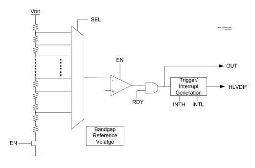
Since the HLVD can be software enabled through the EN bit, setting and clearing the enable bit does not produce a false HLVD event glitch. Each time the HLVD module is enabled, the RDY bit can be used to detect when the module is stable and ready to use.
