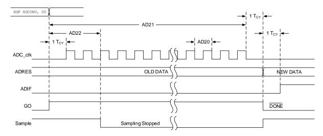
Figure 45-10. ADC Conversion Timing (ADC Clock from ADCRC)
