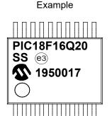
20-Lead SOIC (7.50 mm)
