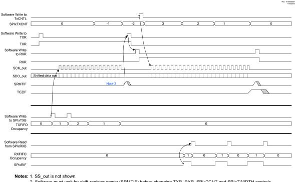
Figure 35-5. SPI Host Operation - Command+Read Data, TXR = 0, RXR = 1
