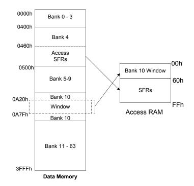
Remapping of the Access Bank applies only to operations using the Indexed Literal Offset mode. Operations that use the BSR (Access RAM bit is '1') will continue to use Direct Addressing as before.
