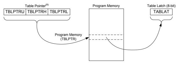
**Note:** 1. The Table Pointer register points to a byte in program memory.
