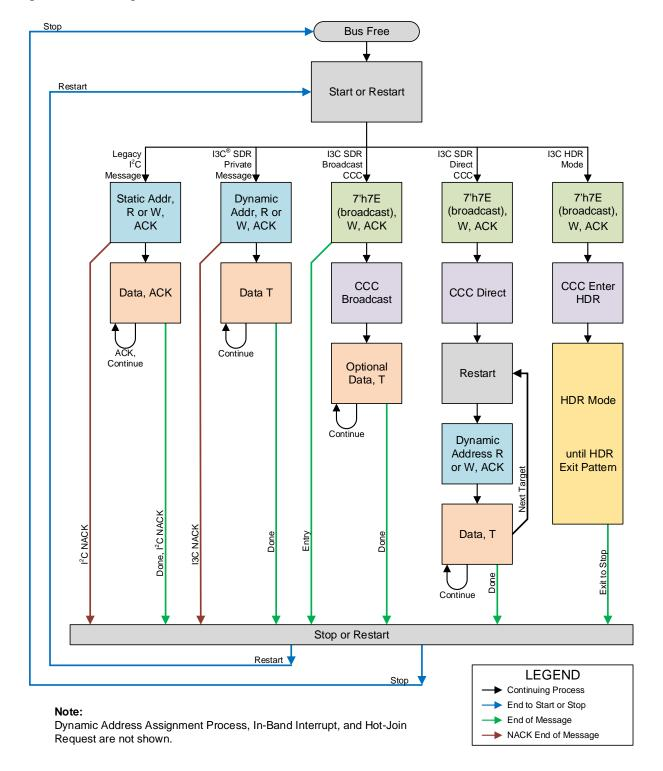
Figure 37-7. I3C® Target Bus Communication Flowchart
