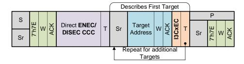
Figure 37-23. Broadcast Write ENEC/DISEC Frame Format
