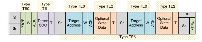
Figure 37-56. Direct CCC Read Error Type Frame Format
