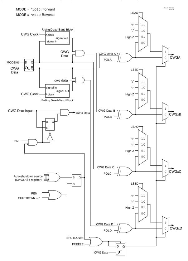
In Forward Full Bridge mode (MODE = <code>\b010</code>), CWGxA is driven to its Active state, CWGxB and CWGxC are driven to their Inactive state, and CWGxD is modulated by the input signal, as shown in Figure 33-7.
