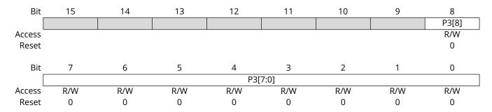
**Bit 8 – P3[8]** Parameter 3 Most Significant bit UART mode operating parameter values
