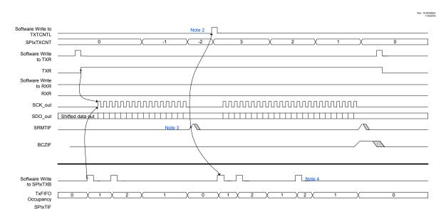
**Figure 35-4.** SPI Host Operation - Command+Write Data, TXR = 1, RXR = 0
