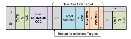
Figure 37-40. Direct Read GETMXDS Frame Format 2
