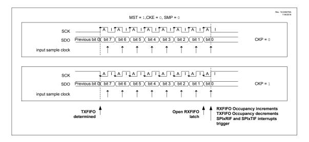
Figure 35-8. Clocking Detail - Host Mode, CKE = 1, SMP = 1
