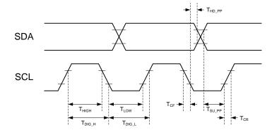
Figure 45-21. I3C Target Out Timing
