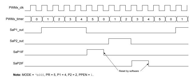
Figure 32-14. Right Aligned Push-Pull Mode Timing Diagram
