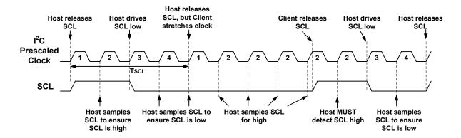
When FME = 2, one SCL period ( $T_{SCL}$ ) is equal to 16 clock periods of the prescaled I2CxCLK source. In other words, the prescaled I2CxCLK source is divided by 16. Using the example from above, if the HFINTOSC (64 MHz) clock source is selected, I2CxBAUD is loaded with a value of '3', and FME = 2, the actual SCL frequency is 1 MHz (see the equation below).
