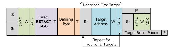
Figure 37-34. Direct Read RSTACT Frame Format
