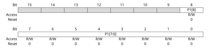
**Bit 8 – P1[8]** Parameter 1 Most Significant bit UART mode operating parameter values
