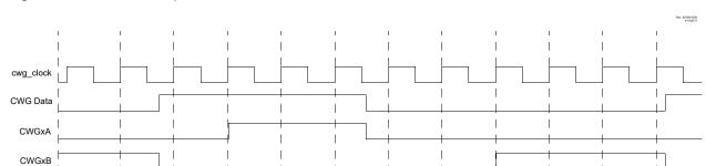
Figure 33-12. Dead-Band Operation, CWGxDBR =  $0 \times 01$ , CWGxDBF =  $0 \times 02$
