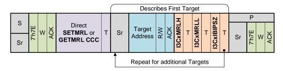
Figure 37-36. Broadcast Write SETMRL Frame Format
