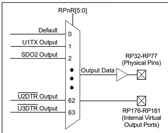
**Note 1:** There are six virtual output ports which are not connected to any I/O ports (RP176-RP181). These virtual ports can be accessed by RPOR17, RPOR18 and RPOR19.
