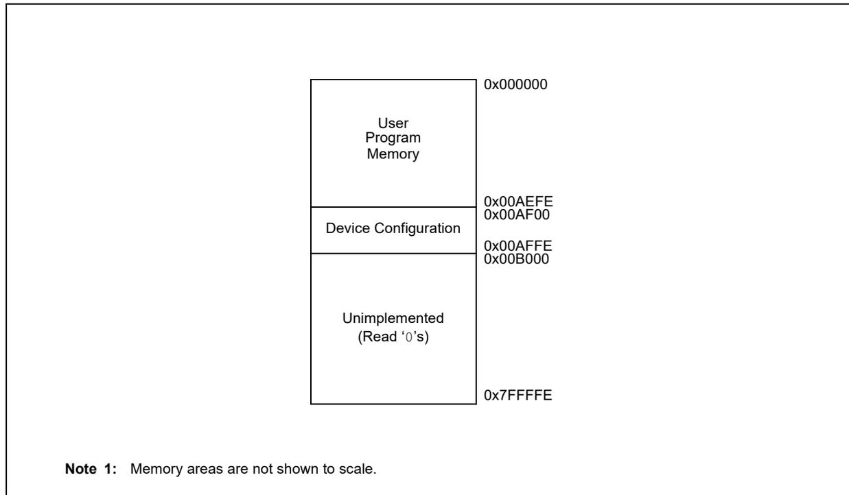
FIGURE 4-3: CODE MEMORY MAP FOR dsPIC33CK32MC10X DEVICES<sup>(1)</sup>
