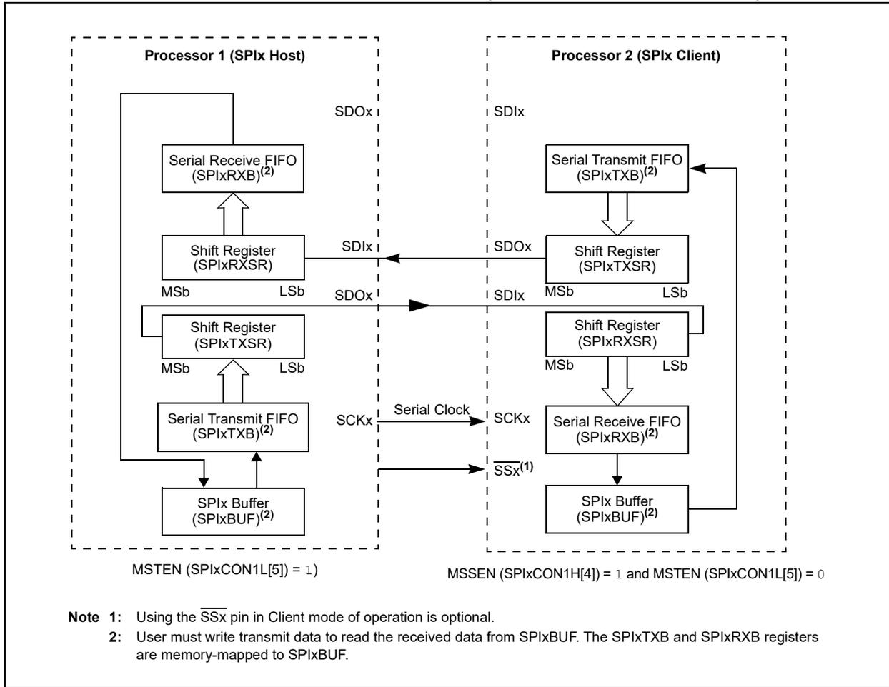
**FIGURE 16-5: SPIx HOST, FRAME HOST CONNECTION DIAGRAM**
