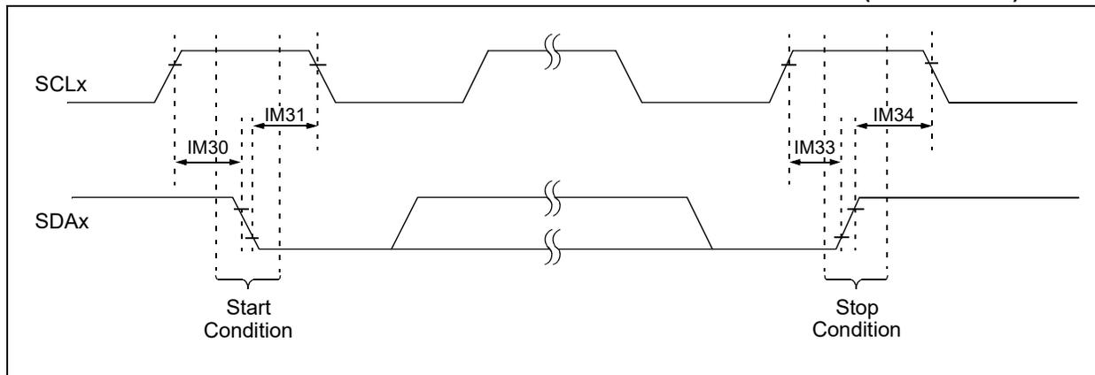
**FIGURE 31-11: I2Cx BUS DATA TIMING CHARACTERISTICS (HOST MODE)**
