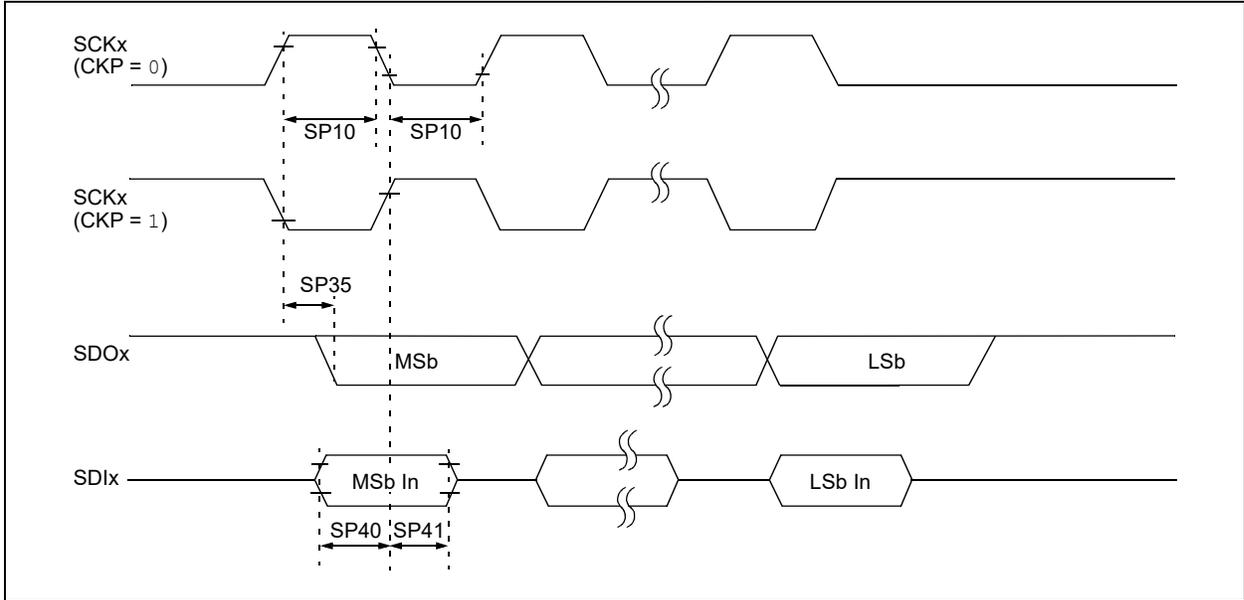
**FIGURE 31-7: SPIx MODULE HOST MODE (CKE = 1) TIMING CHARACTERISTICS**
