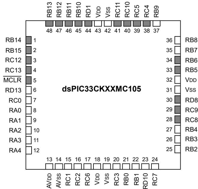
**Legend:** Shaded pins are up to 5VDC tolerant.
