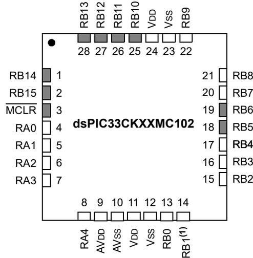
**Legend:** Shaded pins are up to 5 VDC tolerant.
