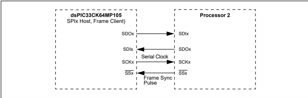
**FIGURE 16-7: SPIx CLIENT, FRAME HOST CONNECTION DIAGRAM**
