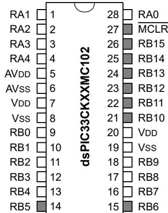
**Legend:** Shaded pins are up to 5 VDC tolerant.
