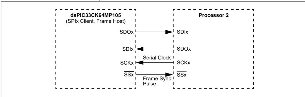
**FIGURE 16-8: SPIx CLIENT, FRAME CLIENT CONNECTION DIAGRAM**
