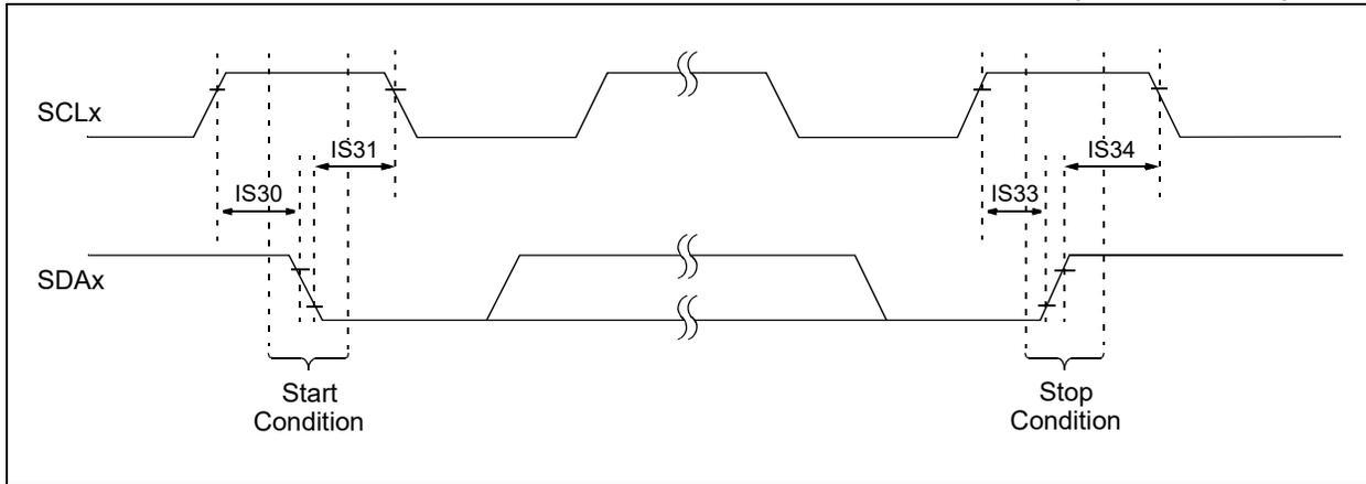
**FIGURE 31-13: I2Cx BUS DATA TIMING CHARACTERISTICS (CLIENT MODE)**
