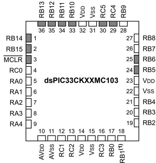
**Legend:** Shaded pins are up to 5 VDC tolerant.
