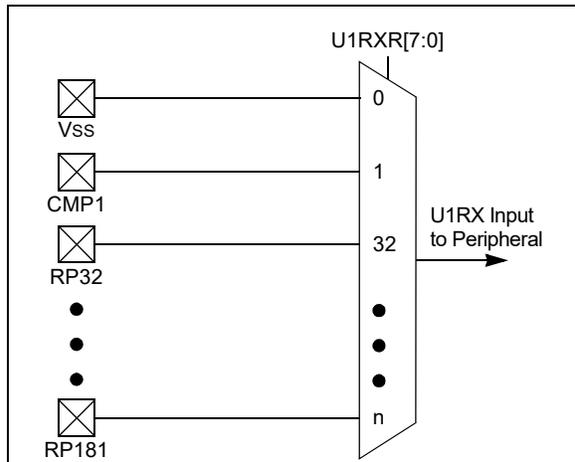
**Note:** For input only, Peripheral Pin Select functionality does not have priority over TRISx settings. Therefore, when configuring an RPn pin for input, the corresponding bit in the TRISx register must also be configured for input (set to '1'). Physical connection to a pin can be made through RP32 through RP77. There are internal signals and virtual pins that can be connected to an input. Table 8-4 shows the details of the input assignment.
