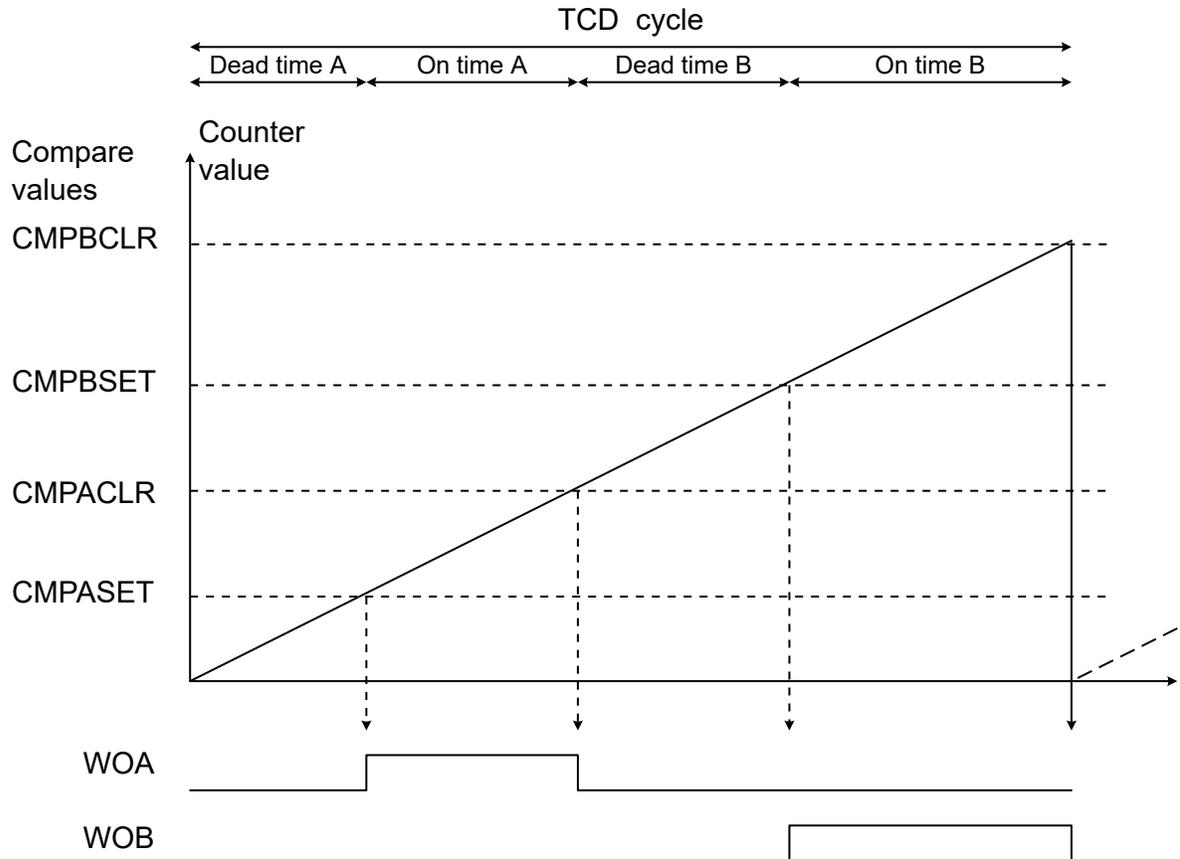
In the figure above,  $\text{CMPASET} < \text{CMPACLR} < \text{CMPBSET} < \text{CMPBCLR}$ . In One Ramp mode, this is required to avoid overlapping outputs during the on time. The figure below is an example where  $\text{CMPBSET} < \text{CMPASET} < \text{CMPACLR} < \text{CMPBCLR}$ , which has overlapping outputs during the on time.
