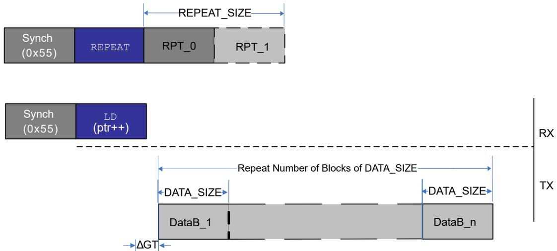
For LD, data will come out continuously after the LD instruction. Note the guard time on the first data block.
