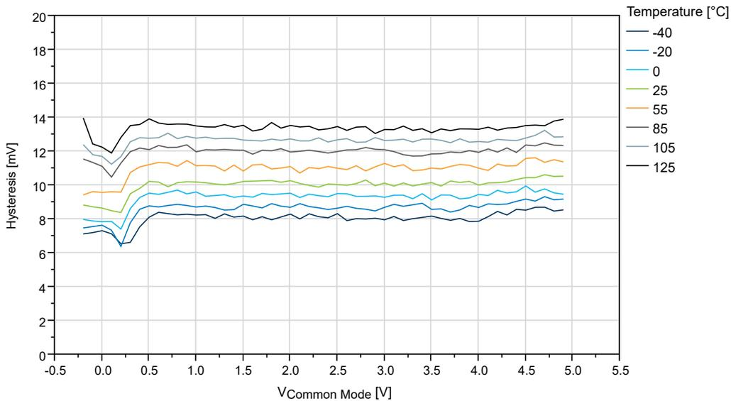
**Figure 36-53. Hysteresis vs.  $V_{CM}$  - 10 mV to 50 mV ( $V_{DD} = 5V$ ,  $T = 25^{\circ}C$ )**
