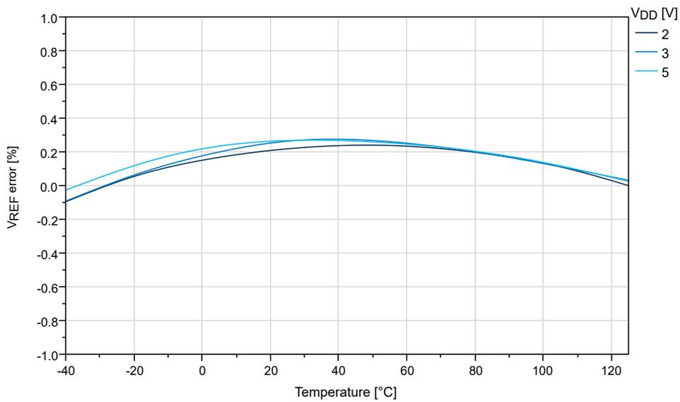
**Figure 36-33. Internal 2.5V Reference vs. Temperature**
