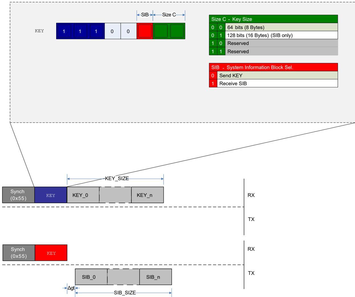
Figure 32-16 shows the transmission of a key and the reception of a SIB. In both cases, the Size C (`SIZE_C`) field in the operand determines the number of frames being sent or received. There is no response after sending a `KEY` to the UPDI. When requesting the SIB, data will be transmitted from the UPDI according to the current guard time setting.
