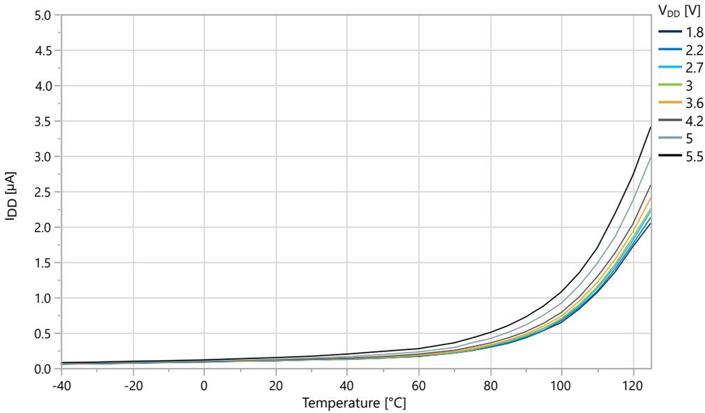
**Figure 36-15. Power-Down Mode Supply Current vs.  $V_{DD}$  (All Functions Disabled)**
