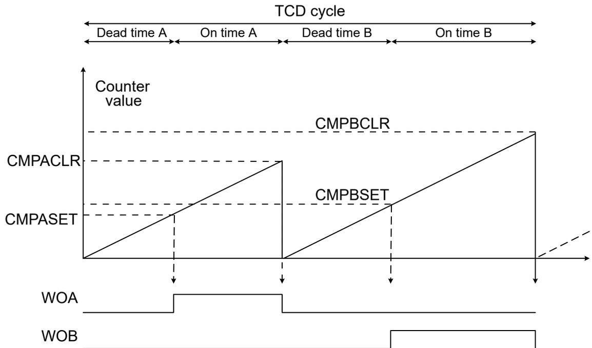
In the figure above,  $CMPASET < CMPACL R$  and  $CMPBSET < CMPBCLR$ . This causes the outputs to go high. There are no restrictions on the  $CMPASET$  and  $CMPACL R$  compared to the  $CMPBSET$  and  $CMPBCLR$  values.
