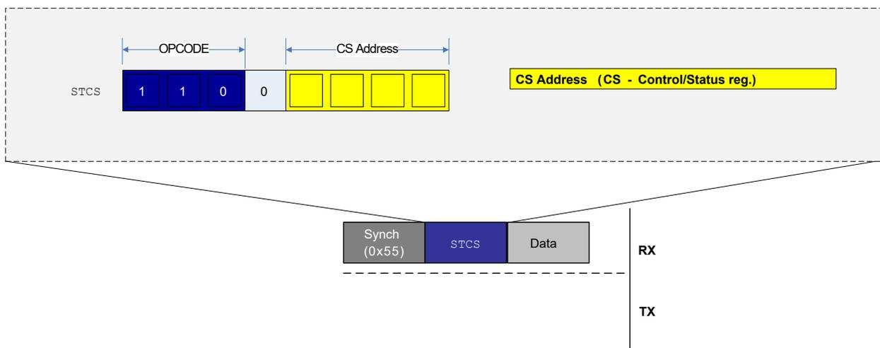
Figure 32-13 shows the data frame transmitted after the SYNCH character and the instruction frames. The STCS instruction byte can be immediately followed by the data byte. There is no response generated from the STCS instruction, as is the case for the ST and STS instructions.
