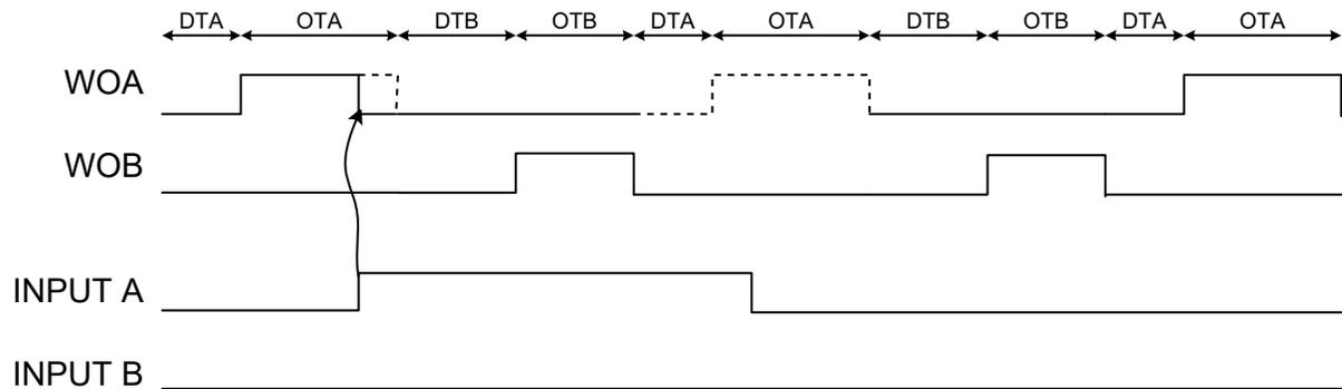
If Input mode 10 is used on input B and an input event occurs, the WOB will be OFF as long as the event lasts. If released during an on time, it will be OFF for the rest of the on time.
