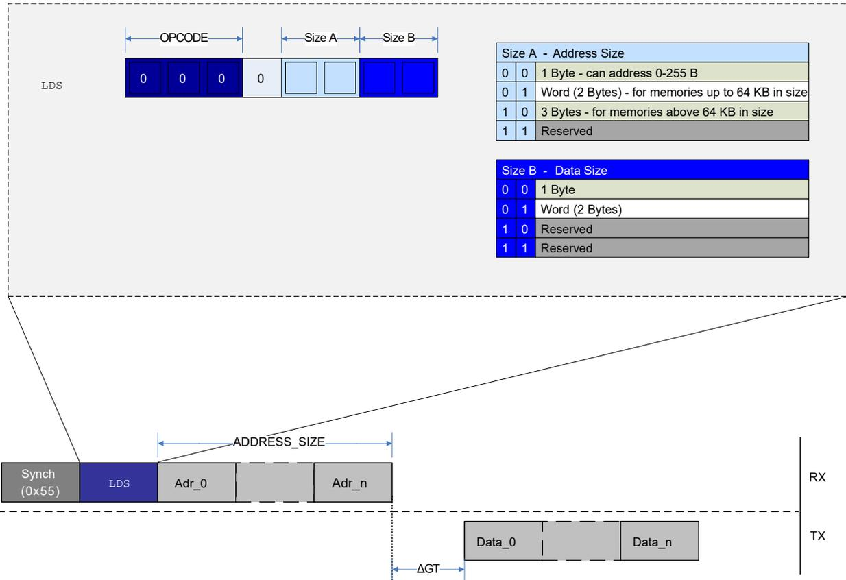
When the instruction is decoded, and the address byte(s) are received as dictated by the decoded instruction, the DL layer will synchronize all required information to the ACC layer, which will handle the bus request and synchronize data buffered from the bus back again to the DL layer. This will create a synchronization delay that must be taken into consideration upon receiving the data from the UPDI.
