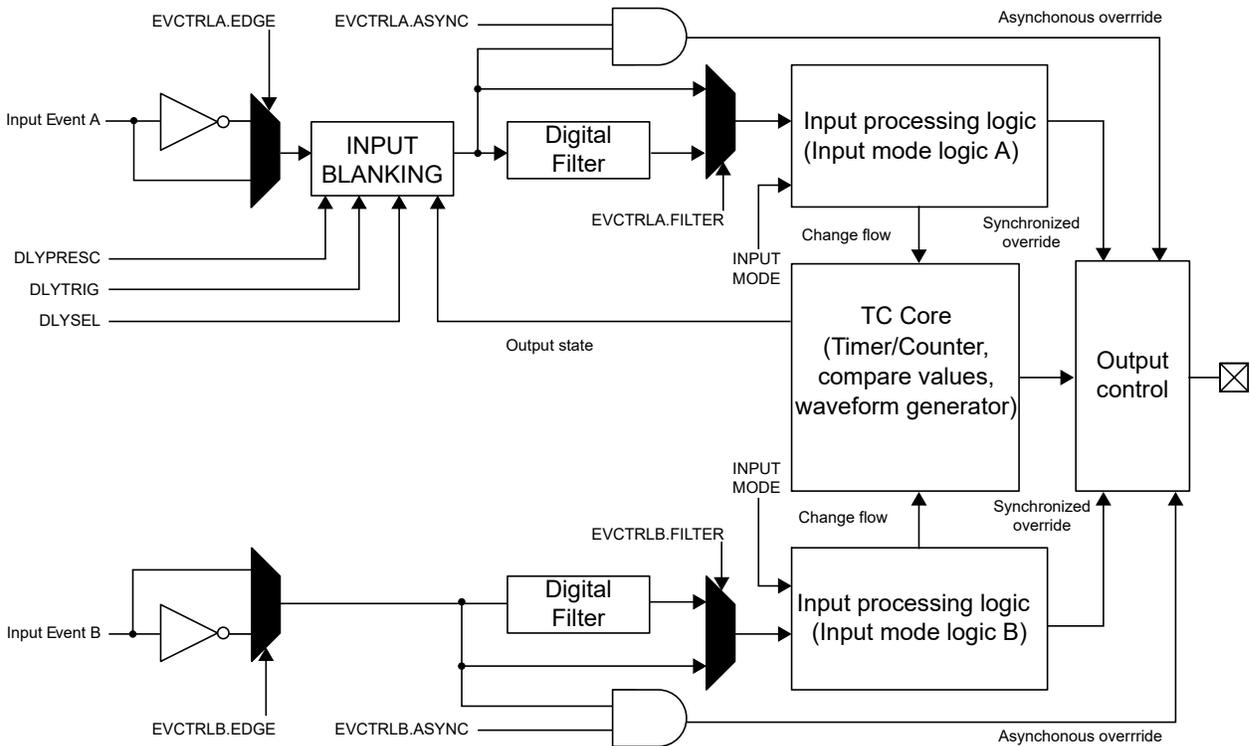
There is a delay of two/three clock cycles on the TCD synchronizer clock between receiving the input event, processing it, and overriding the outputs. If using the asynchronous event detection, the outputs will override instantly outside the input processing.
