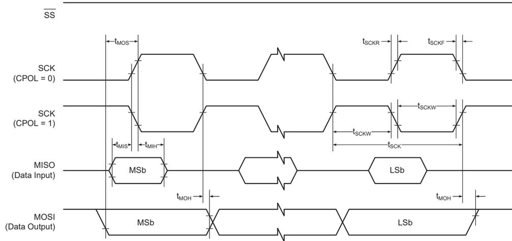
Figure 35-6. SPI - Timing Requirements in Client Mode
