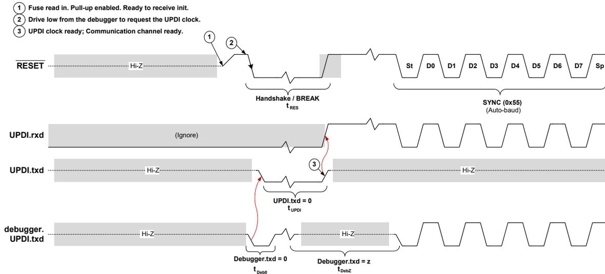
When the negative edge is detected, the UPDI clock starts. The UPDI will continue to drive the line low until the clock is stable and ready for the UPDI to use. The duration of  $t_{UPDI}$  will vary, depending on the status of the oscillator when the UPDI is enabled. After this duration, the data line will be released by the UPDI and pulled high.
