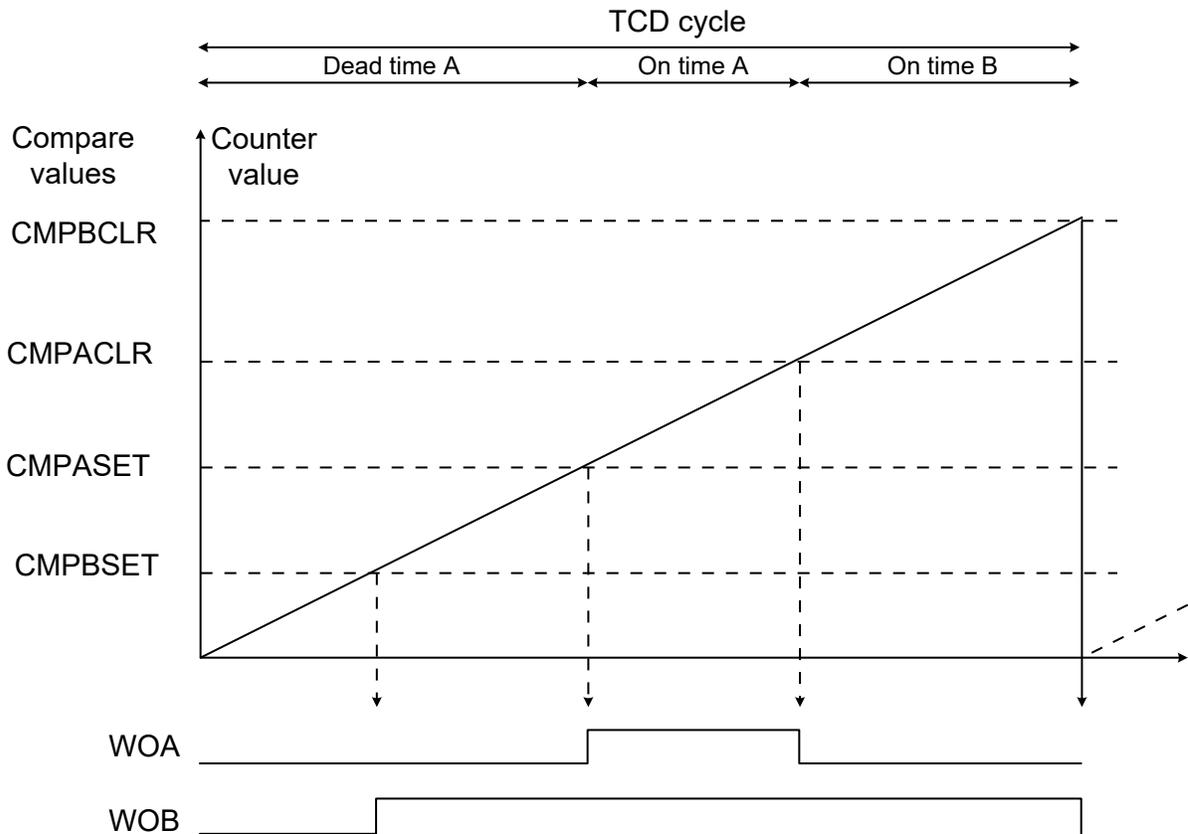
A match with  $CMPBCLR$  will always result in all outputs being cleared. If any of the other compare values are bigger than  $CMPBCLR$ , their associated effect will never occur. If the  $CMPACLR$  is smaller than the  $CMPASET$  value, the clear value will not have any effect.
