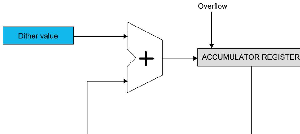
The user can select where in the TCD cycle the dither will be added by writing to the Dither Selection (DITHERSEL) bits in the Dither Control (TCDn.DITCTRL) register:
