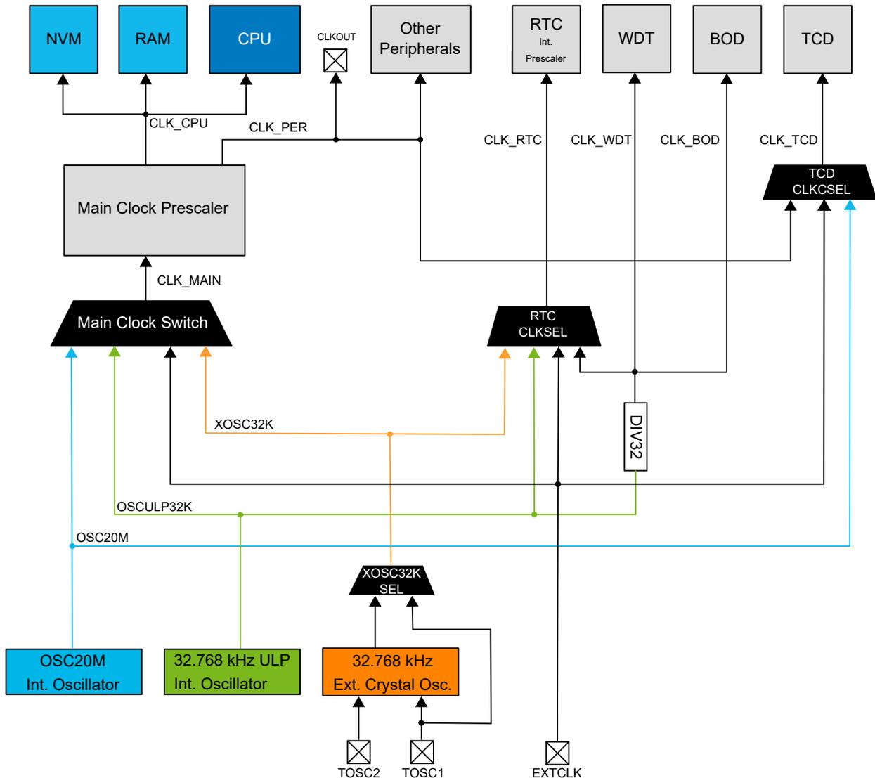
**Note:** The availability of the TOSC1, TOSC2 and the CLKOUT pin depends on the pin count of the device. See section 5. [I/O Multiplexing and Considerations](#) for an overview of which pins are available for each device represented in this data sheet.
