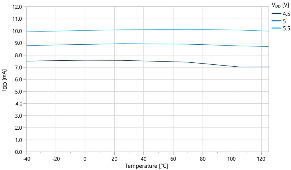
**Figure 36-4. Active Supply Current vs. V<sub>DD</sub> (f = [1.25, 20] MHz OSC20M) at T = 25°C**
