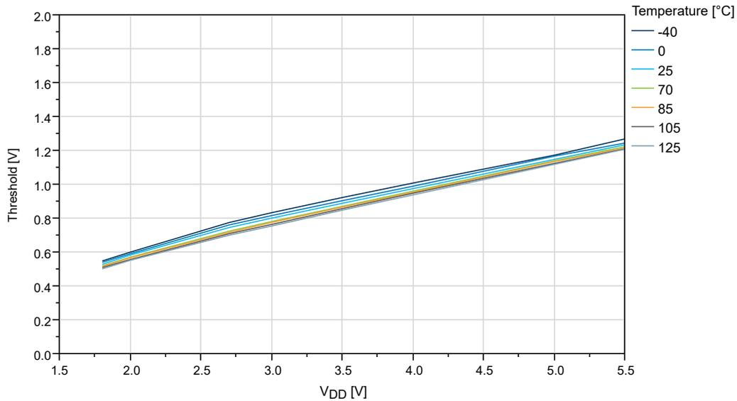
**Figure 36-17. I/O Pin Input Threshold Voltage vs.  $V_{DD}$  ( $T = 25^{\circ}\text{C}$ )**
