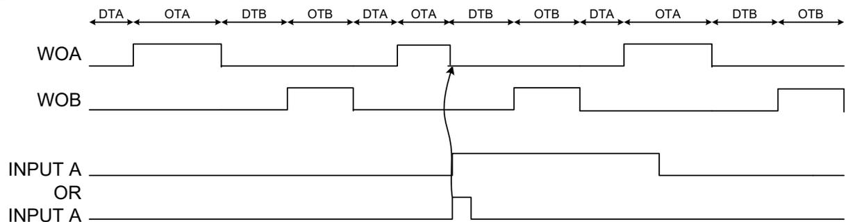
If Input mode 8 is used on input B and a positive edge on the input event occurs while in on time B, the TCD counter jumps to dead time A.
