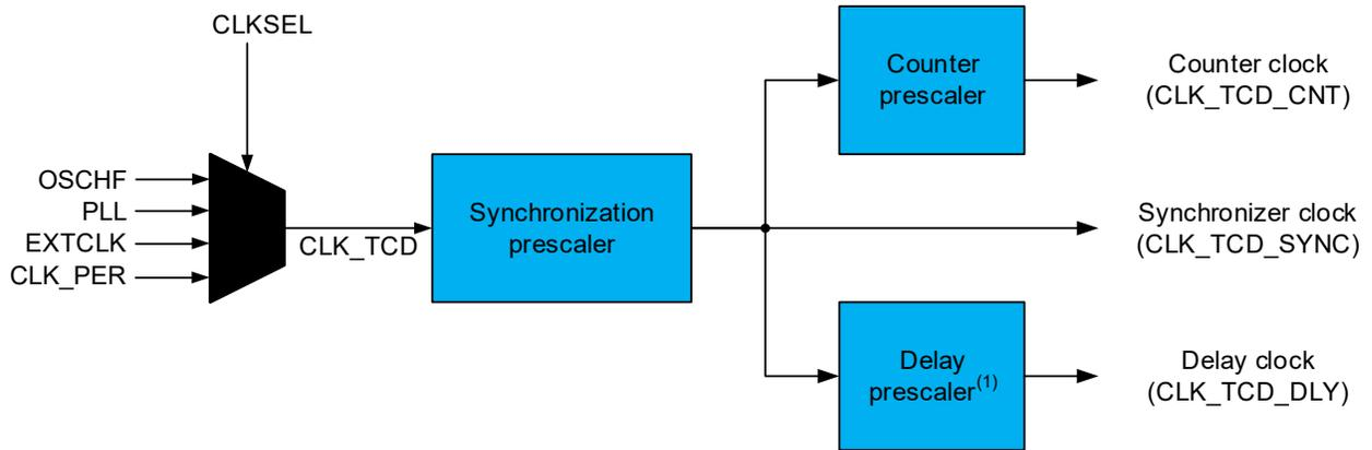
1. Used by input blanking/delay event out.
