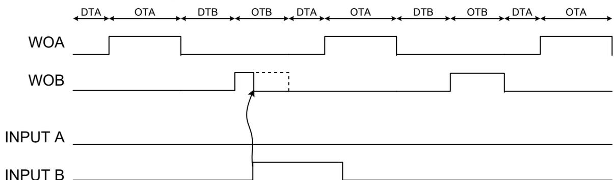
**Input Mode 10: Stop Output at Level, Maintain Frequency**
