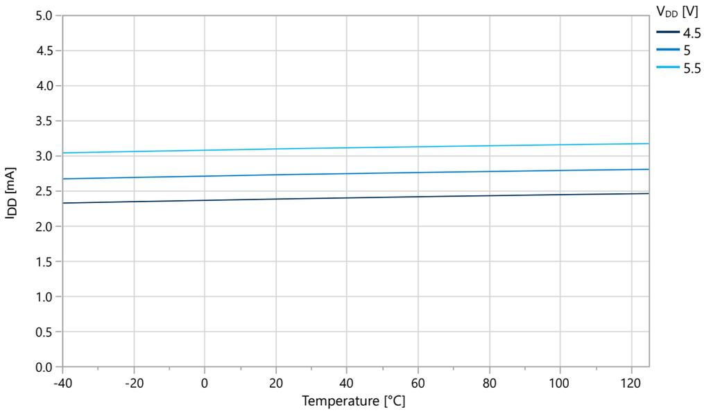
**Figure 36-9. Idle Supply Current vs.  $V_{DD}$  ( $f = 32.768$  kHz OSCULP32K)**
