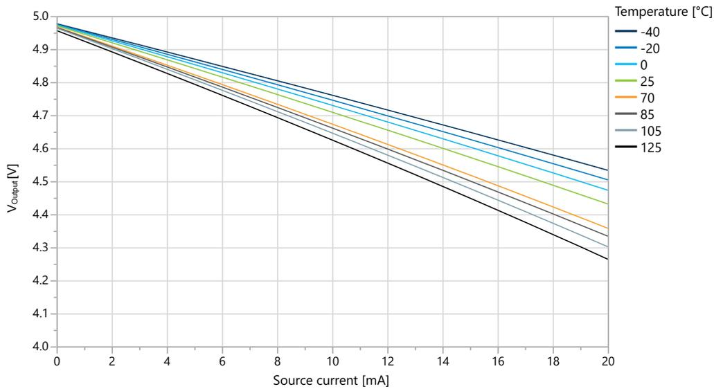
Figure 36-27. I/O Pin Output Voltage vs. Source Current (T = 25°C)
