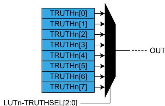
Configure the truth table inputs (LUTn-TRUTHSEL[2:0]) by writing the Input Source Selection bit fields in the LUT Control registers:
