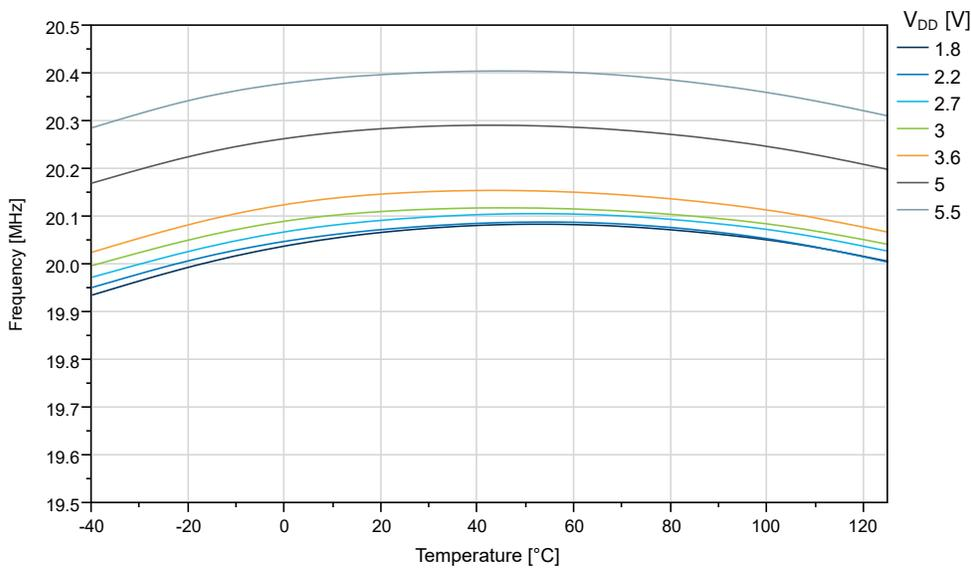
**Figure 36-63. OSC20M Internal Oscillator: Frequency vs.  $V_{DD}$**
