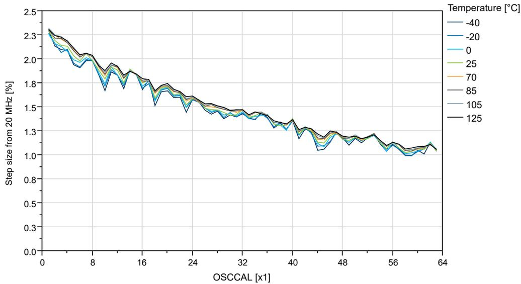
**Figure 36-61. OSC20M Internal Oscillator: Frequency vs. Calibration Value ( $V_{DD} = 3V$ )**
