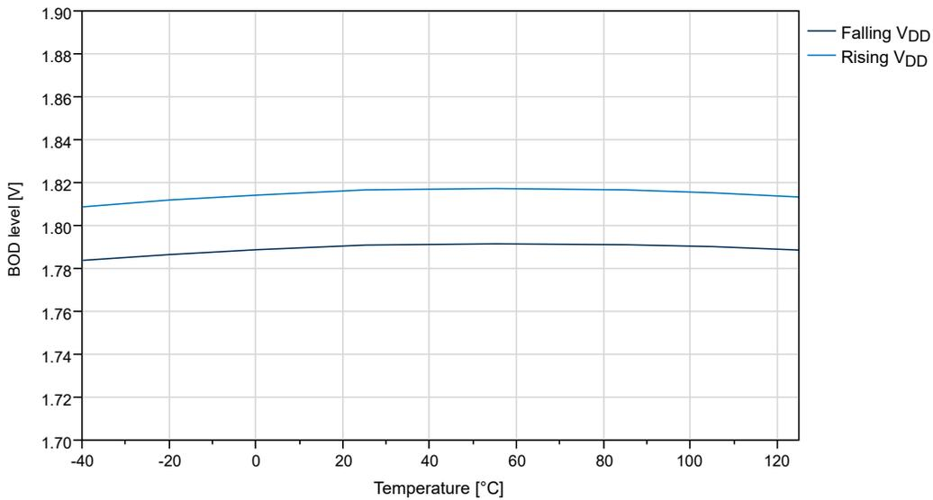
**Figure 36-39. BOD Threshold vs. Temperature (Level 2.6V)**
