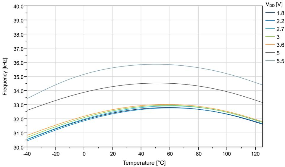
**Figure 36-65. OSCULP32K Internal Oscillator Frequency vs.  $V_{DD}$**
