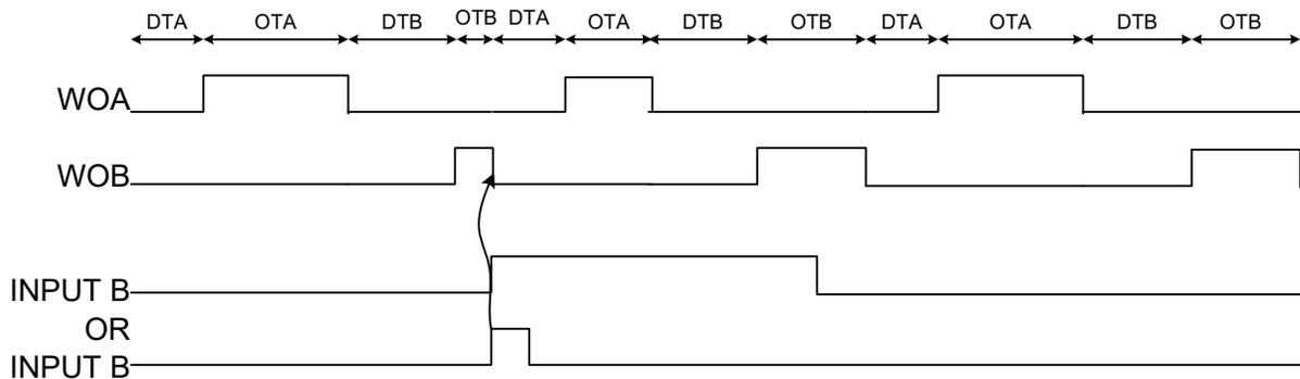
**Input Mode 9: Stop Output on Edge, Maintain Frequency**
