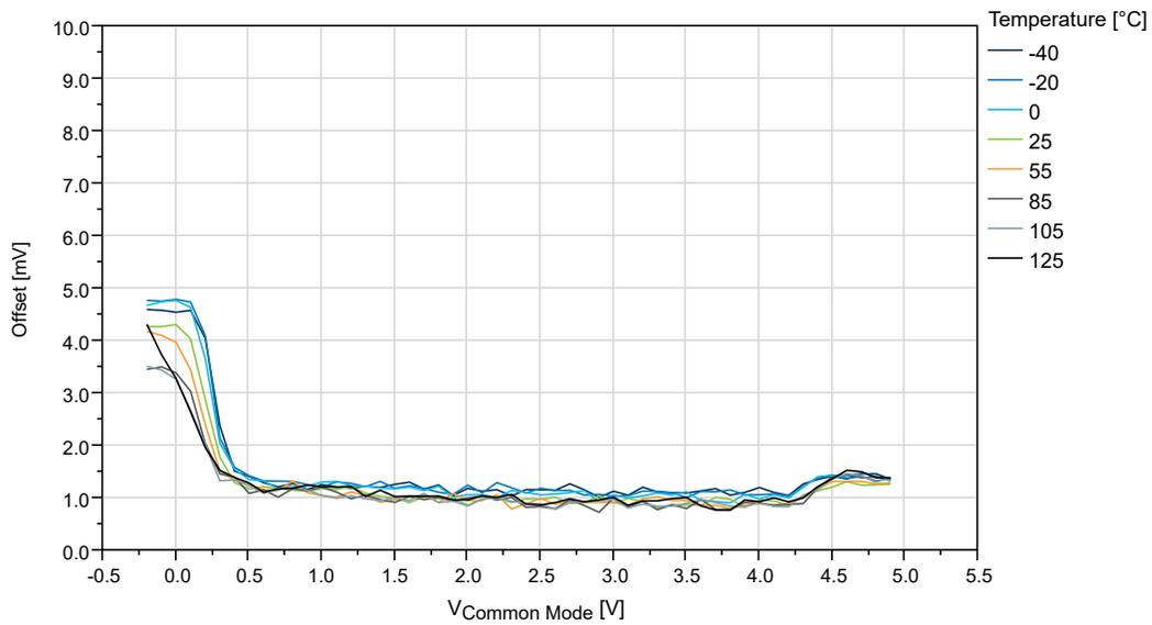
**Figure 36-55. Offset vs.  $V_{CM}$  - 10 mV to 50 mV ( $V_{DD} = 5V$ ,  $T = 25^{\circ}C$ )**
