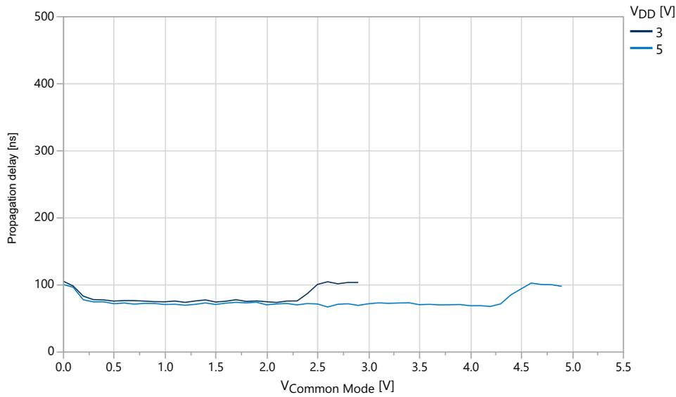
**Figure 36-57. Propagation Delay vs.  $V_{CM}$  LPMODE Enabled, Rising Positive Input,  $V_{OD} = 30$  mV ( $T = 25^\circ\text{C}$ )**
