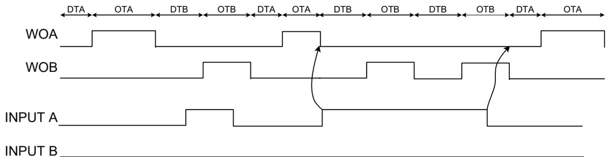
If Input mode 3 is used on input B, an event will only have an effect if the TCD is in dead time B or on time B.
