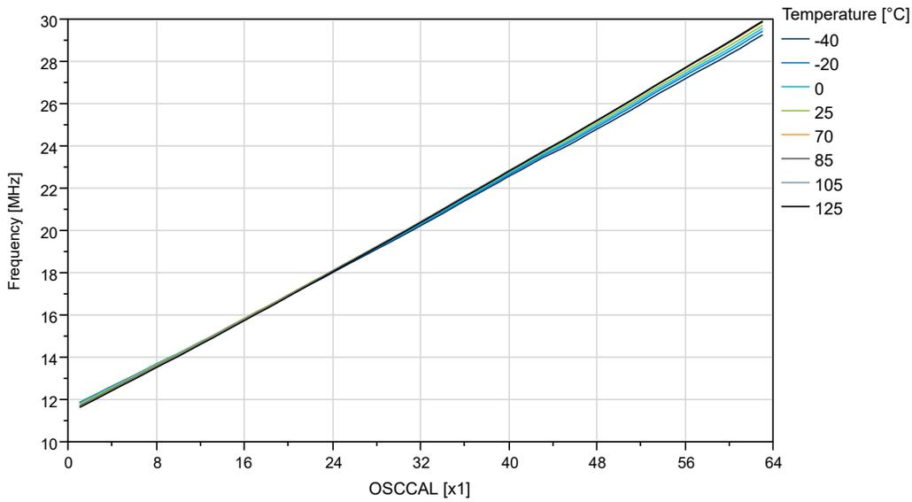
**Figure 36-62. OSC20M Internal Oscillator: Frequency vs. Temperature**
