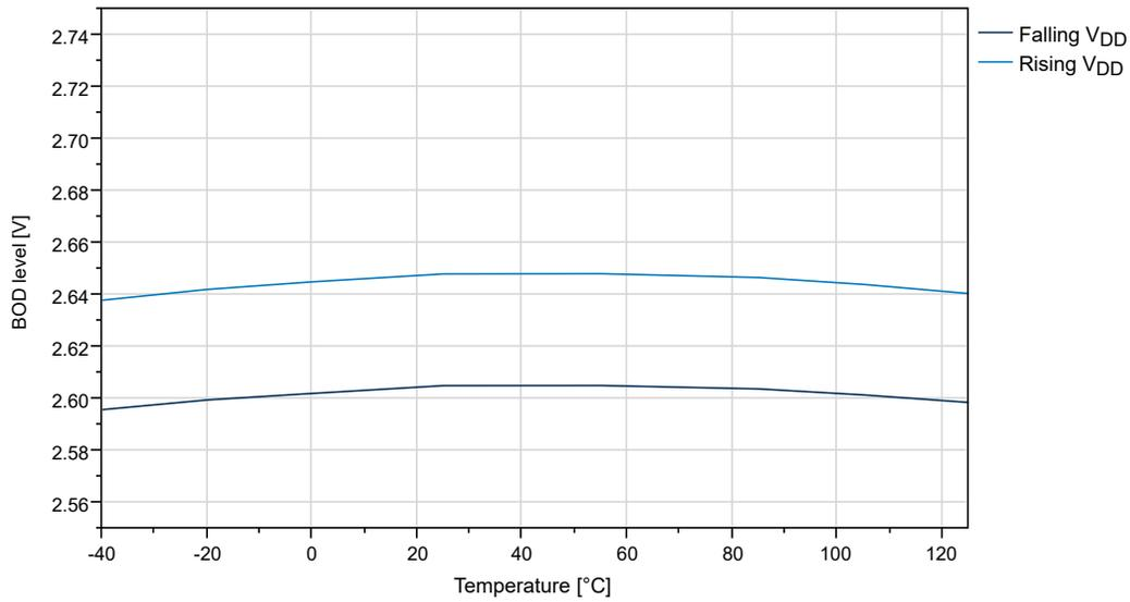
**Figure 36-40. BOD Threshold vs. Temperature (Level 4.3V)**
