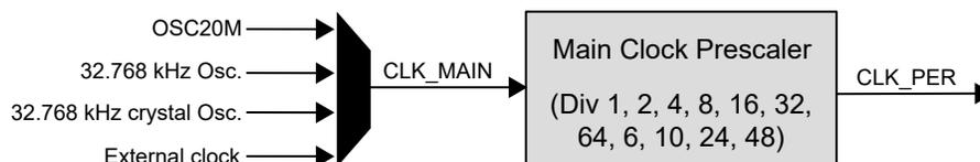
The Main Clock and Prescaler configuration (CLKCTRL.MCLKCTRLA, CLKCTRL.MCLKCTRLB) registers are protected by the Configuration Change Protection Mechanism, employing a timed write procedure for changing these registers.
