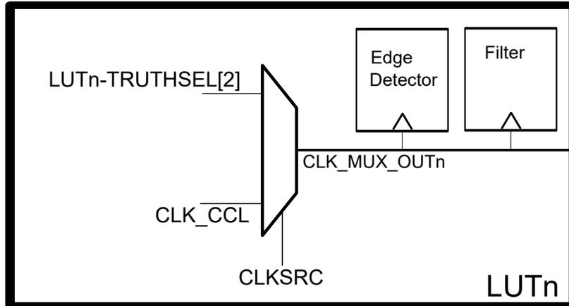
When the CLKSRC bit is written to 0x1, LUTn-TRUTHSEL[2] is used to clock the corresponding filter and edge detector (CLK\_MUX\_OUTn). The sequencer is clocked by the CLK\_MUX\_OUTn of the even LUT in the pair. When CLKSRC is written to 0x1, LUTn-TRUTHSEL[2] is treated as OFF (low) in the truth table.
