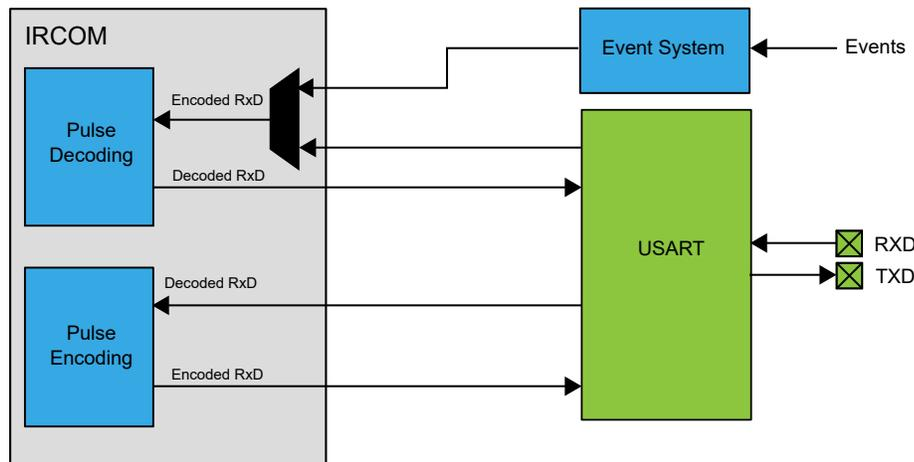
The USART is set in IRCOM mode by writing `0x02` to the CMODE bit field in the USARTn.CTRLC register. The data on the TXD/RXD pins are the inverted values of the transmitted/received infrared pulse. It is also possible to select an event channel from the Event System as an input for the IRCOM receiver. This enables the IRCOM to receive input from the I/O pins or sources other than the corresponding RXD pin, which will disable the RxD input from the USART pin.
