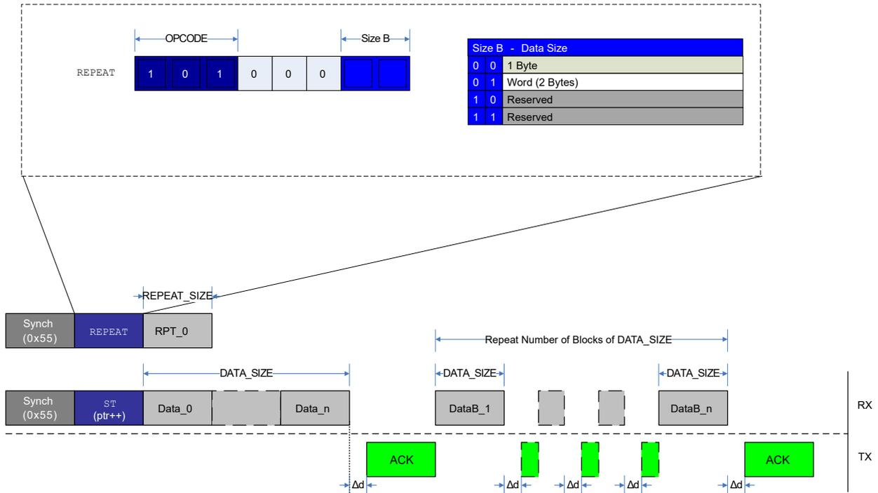
Figure 32-14 gives an example of a repeat operation with an ST instruction using pointer post-increment operation. After the REPEAT instruction is sent with  $RPT\_0 = n$ , the first ST instruction is issued with SYNCH and instruction frame, while the next  $n$  ST instructions are executed by only sending data bytes according to the ST operand DATA\_SIZE, and maintaining the Acknowledge (ACK) handshake protocol.
