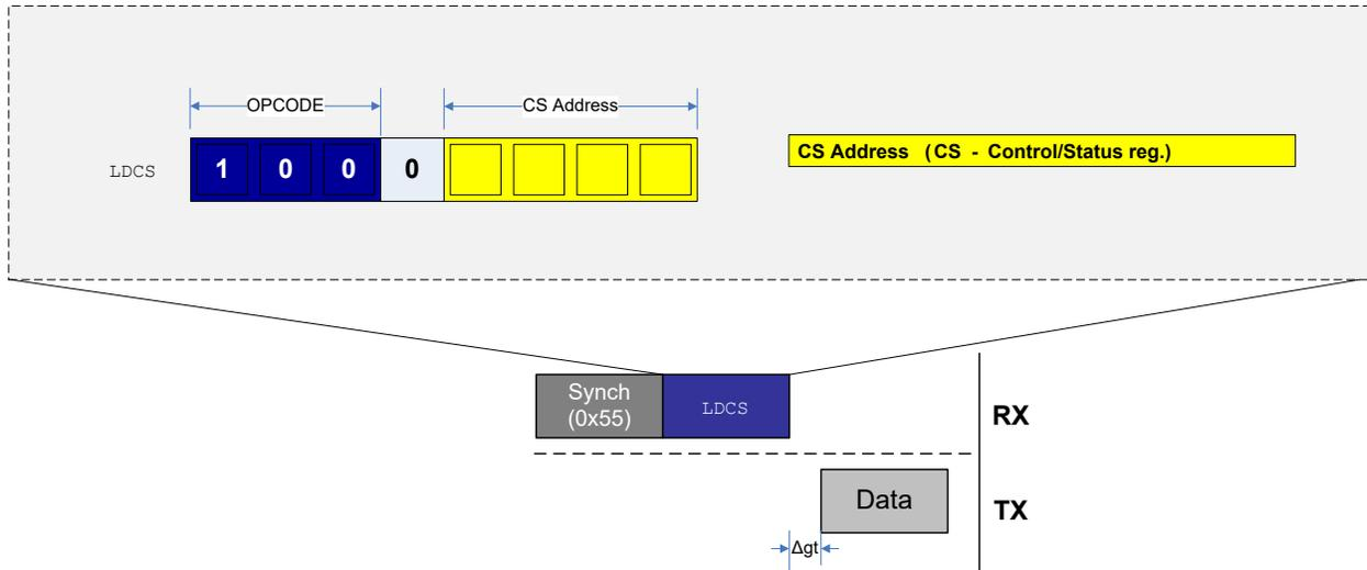
Figure 32-12 shows a typical example of `LDCS` data transmission. A data byte from the `LDCS` is transmitted from the UPDI after the guard time is completed.
