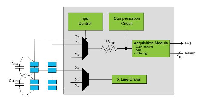
Figure 31-2. PTC Block Diagram Self-Capacitance
