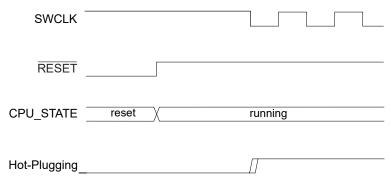
The presence of a debugger probe is detected when either Hot-Plugging or Cold-Plugging is detected. Once detected, the Debugger Present bit of the Status B register (STATUSB.DBGPRES) is set. For security reasons, Hot-Plugging is not available when the device is protected by the NVMCTRL security bit.
