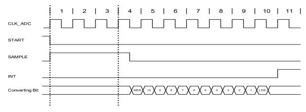
Figure 28-5. ADC Timing for Free Running in Differential Mode without Gain
