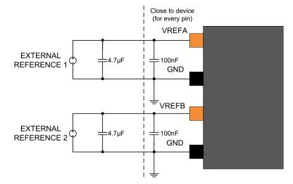
Figure 36-3. External Analog Reference Schematic With One Reference
