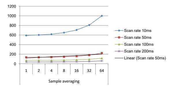
Figure 32-10. Power Consumption [ $\mu$ A] 10 sensors, noise countermeasures Enabled, f=48MHz, Vcc=3.3V
