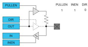
**Note:** When pull is enabled, the pull value is defined by the OUT value.
