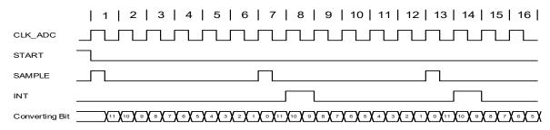
Figure 28-6. ADC Timing for One Conversion in Single-Ended Mode without Gain
