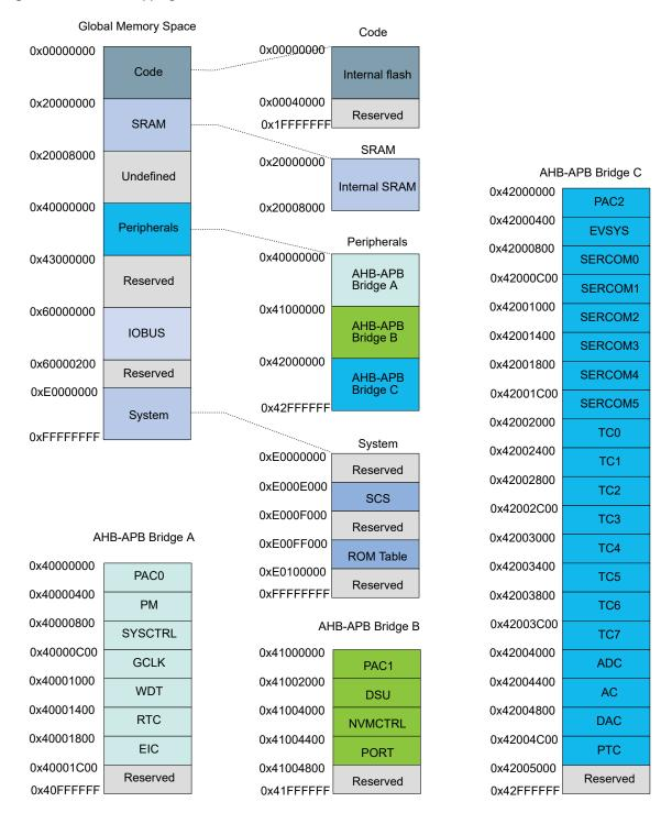
This figure represents the full configuration of the SAM D20 device with maximum flash and SRAM capabilities and a full set of peripherals. Refer to the Configuration Summary for details.
