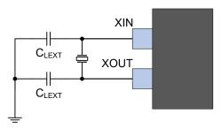
The crystal should be located as close to the device as possible. Long signal lines may cause a load too high to operate the crystal, and cause crosstalk to other parts of the system.
