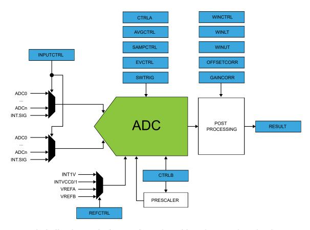
**Note:** INT1V is the buffered internal reference of 1.0V, derived from the internal 1.1V bandgap reference.
