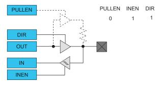
Figure 21-8. I/O Configuration - Output with Pull
