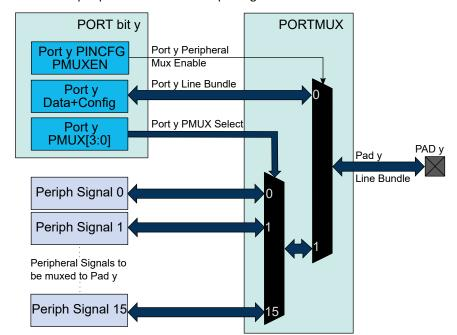
Figure 21-3. Overview of the peripheral functions multiplexing
