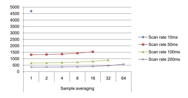
Figure 32-12. Power Consumption [ $\mu$ A] 100 sensors, noise countermeasures Enabled, f=48MHz, Vcc=3.3V
