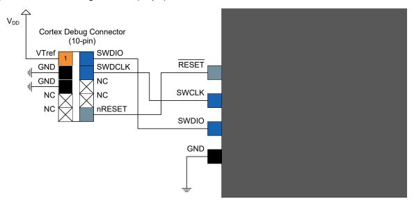
Table 36-9. Cortex Debug Connector (10-pin)
