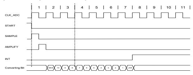
Figure 28-7. ADC Timing for Free Running in Single-Ended Mode without Gain
