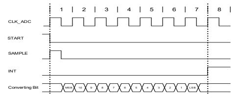
The sampling time can be increased by using the Sampling Time Length bit group in the Sampling Time Control register (SAMPCTRL.SAMPLEN). As example, the next figure is showing the timing conversion.
