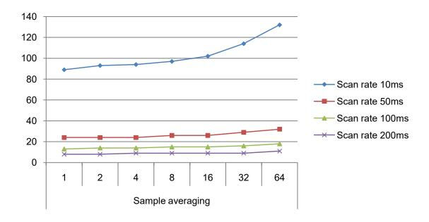
**Figure 32-8.** Power Consumption [μA] 1 sensor, noise countermeasures Enabled, f=48MHz, Vcc=3.3V
