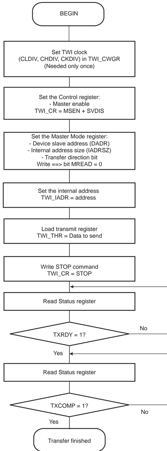
Figure 34-16. TWI Write Operation with Multiple Data Bytes with or without Internal Address
