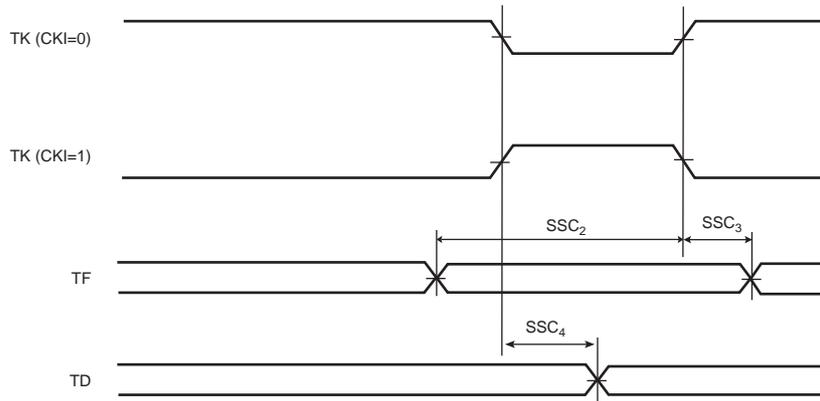
**Figure 44-29. SSC Transmitter, TK and TF as Input**
