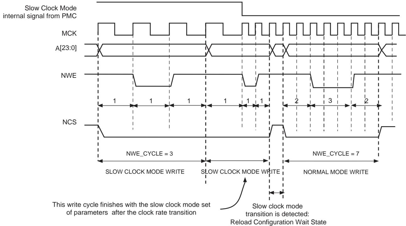
**Figure 26-30. Recommended Procedure to Switch from Slow Clock Mode to Normal Mode or from Normal Mode to Slow Clock Mode**
