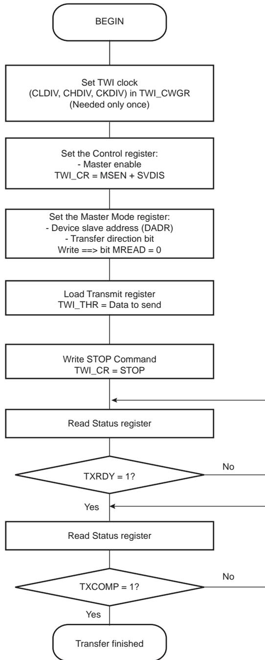
**Figure 34-15. TWI Write Operation with Single Data Byte and Internal Address**
