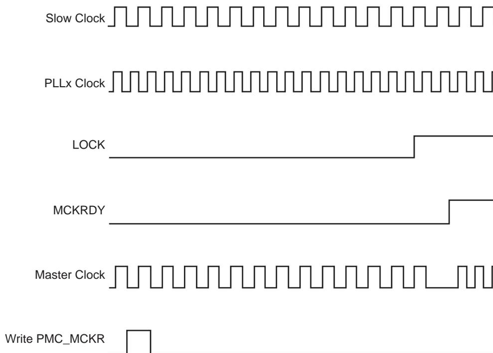
**Figure 29-7. Switch Master Clock from Main Clock to Slow Clock**
