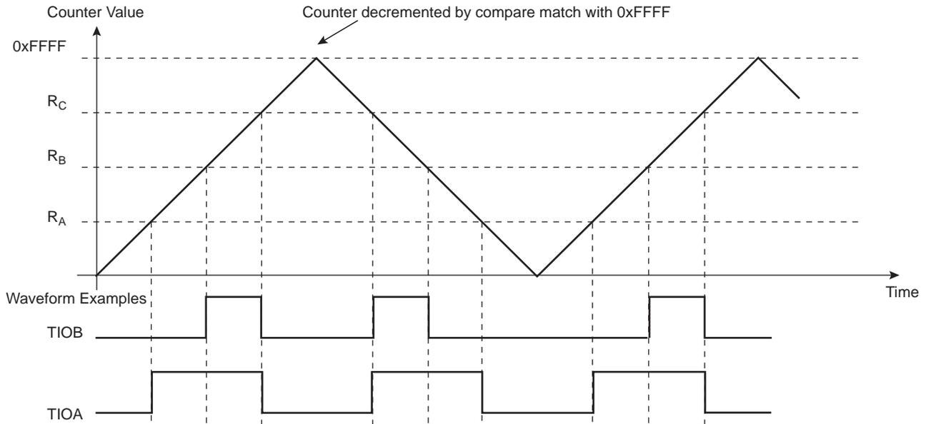
**Figure 37-12. WAVSEL = 01 with Trigger**
