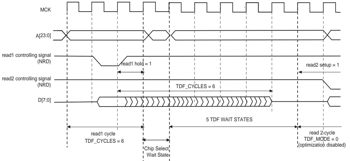
**Figure 26-21. TDF Mode = 0: TDF wait states between a read and a write access on different chip selects**
