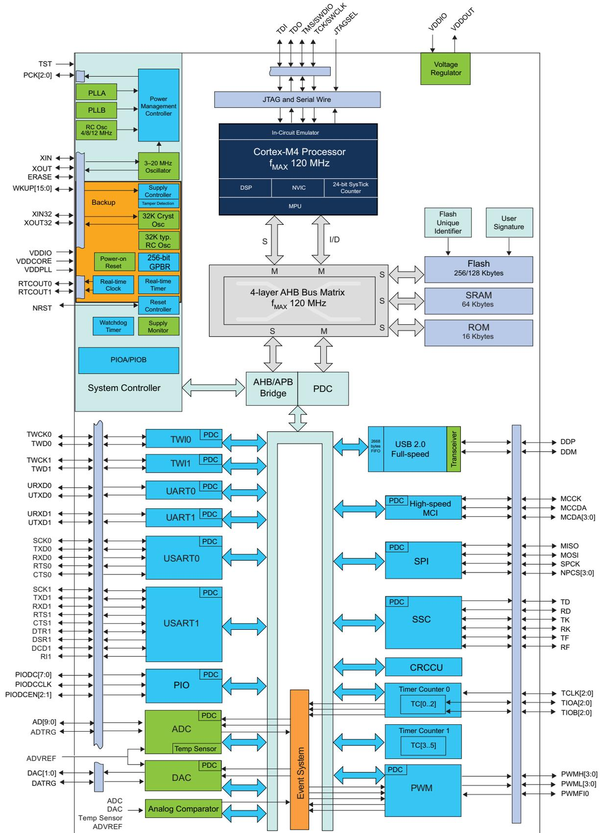
Figure 2-7. SAM4S4/S2 48-pin Version Block Diagram
