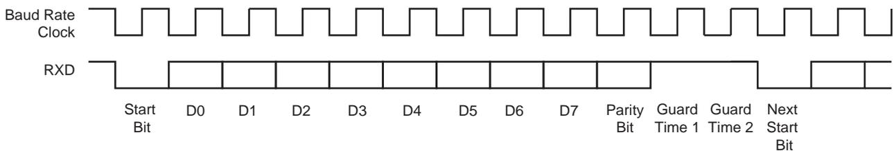
**Figure 36-31. T = 0 Protocol with Parity Error**
