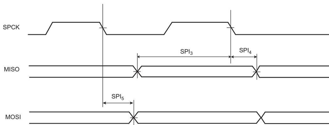
**Figure 44-24. SPI Slave Mode with (CPOL = 0 and NCPHA = 1) or (CPOL = 1 and NCPHA = 0)**
