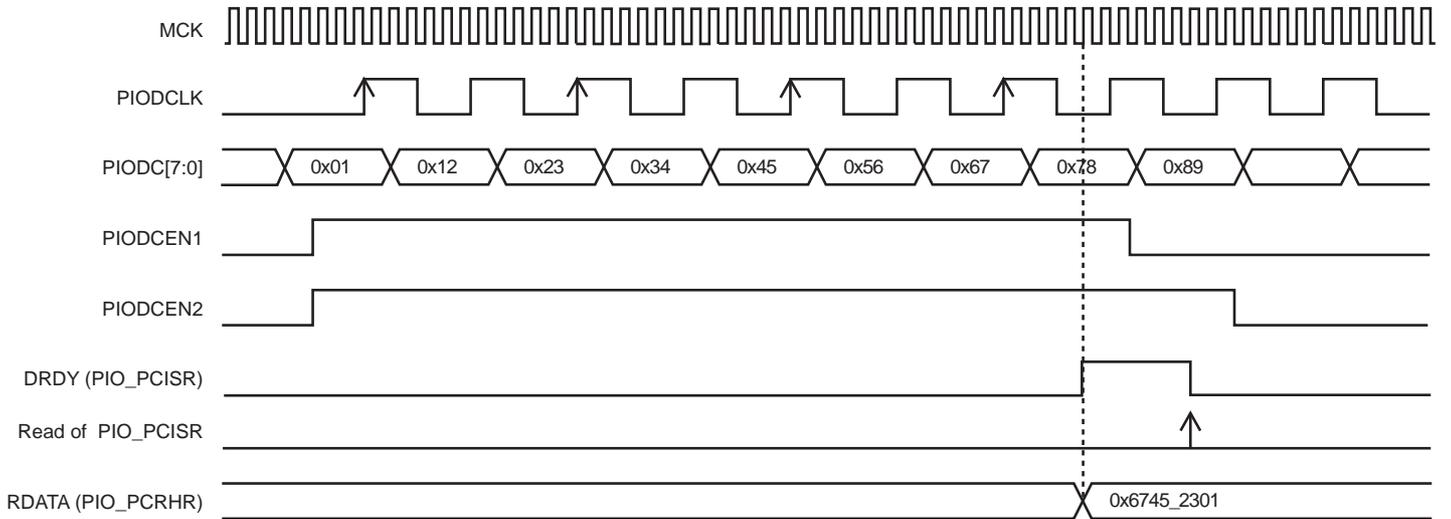
**Figure 31-12. Parallel Capture Mode Waveforms (DSIZE = 2, ALWAYS = 0, HALFS = 1, FRSTS = 1)**
