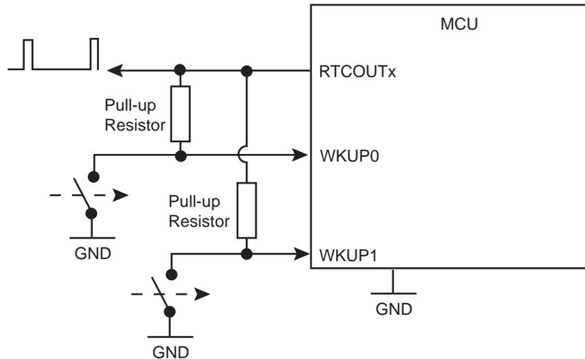
**Figure 18-7. Low-power Debouncer (Push-to-Break Switch, Pull-down Resistors)**
