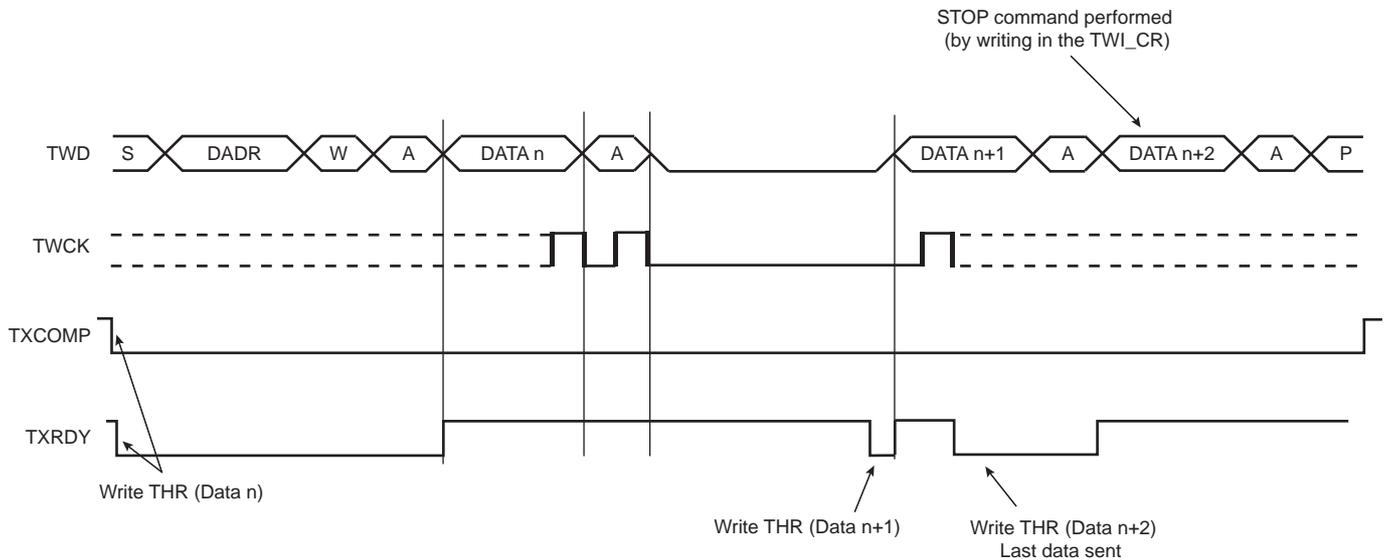
**Figure 34-7. Master Write with One Byte Internal Address and Multiple Data Bytes**
