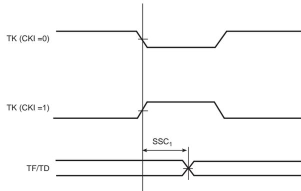
**Figure 44-28. SSC Transmitter, TK as Output and TF as Input**
