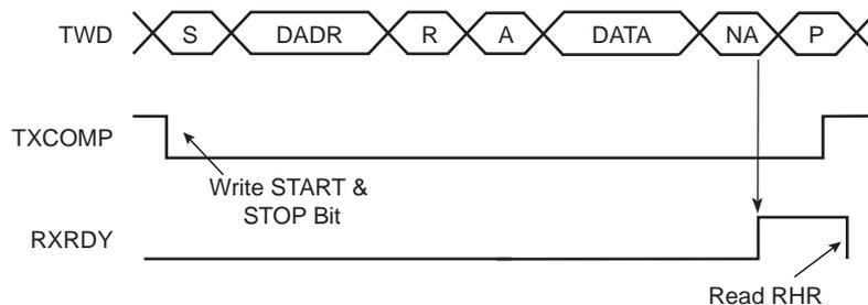
**Figure 34-9. Master Read with Multiple Data Bytes**
