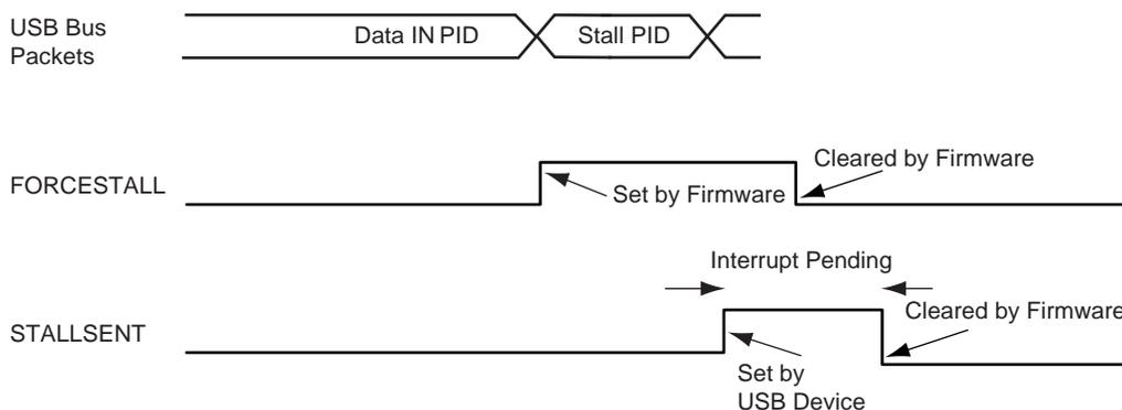
**Figure 40-13. Stall Handshake (Data OUT Transfer)**
