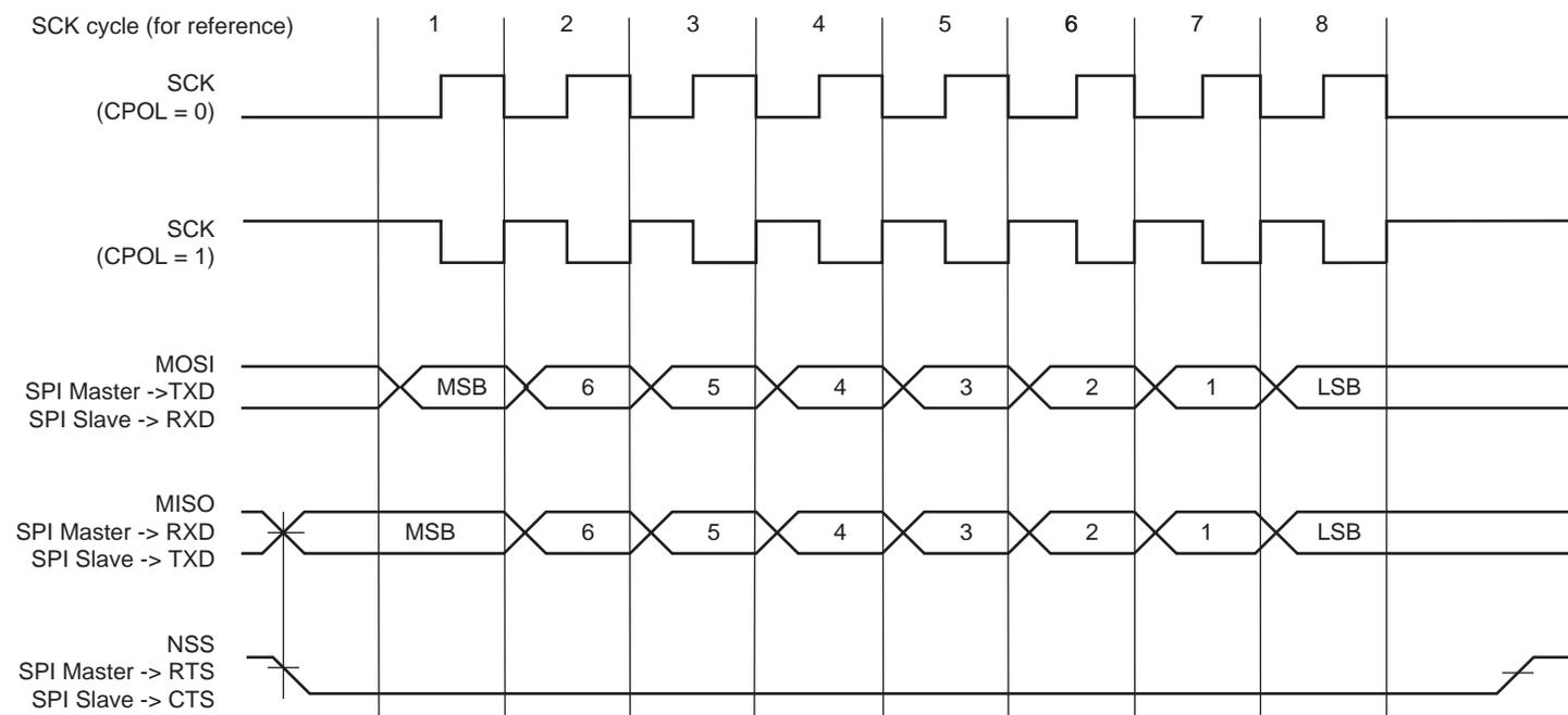
**Figure 36-38. SPI Transfer Format (CPHA = 0, 8 bits per transfer)**
