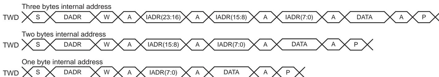
**Figure 34-11. Master Read with One, Two or Three Bytes Internal Address and One Data Byte**
