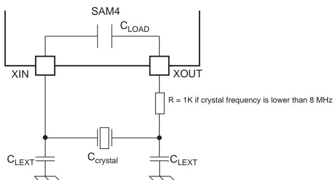
$$C_{LEXT} = 2 \times (C_{crystal} - C_{LOAD} - C_{PCB}).$$
