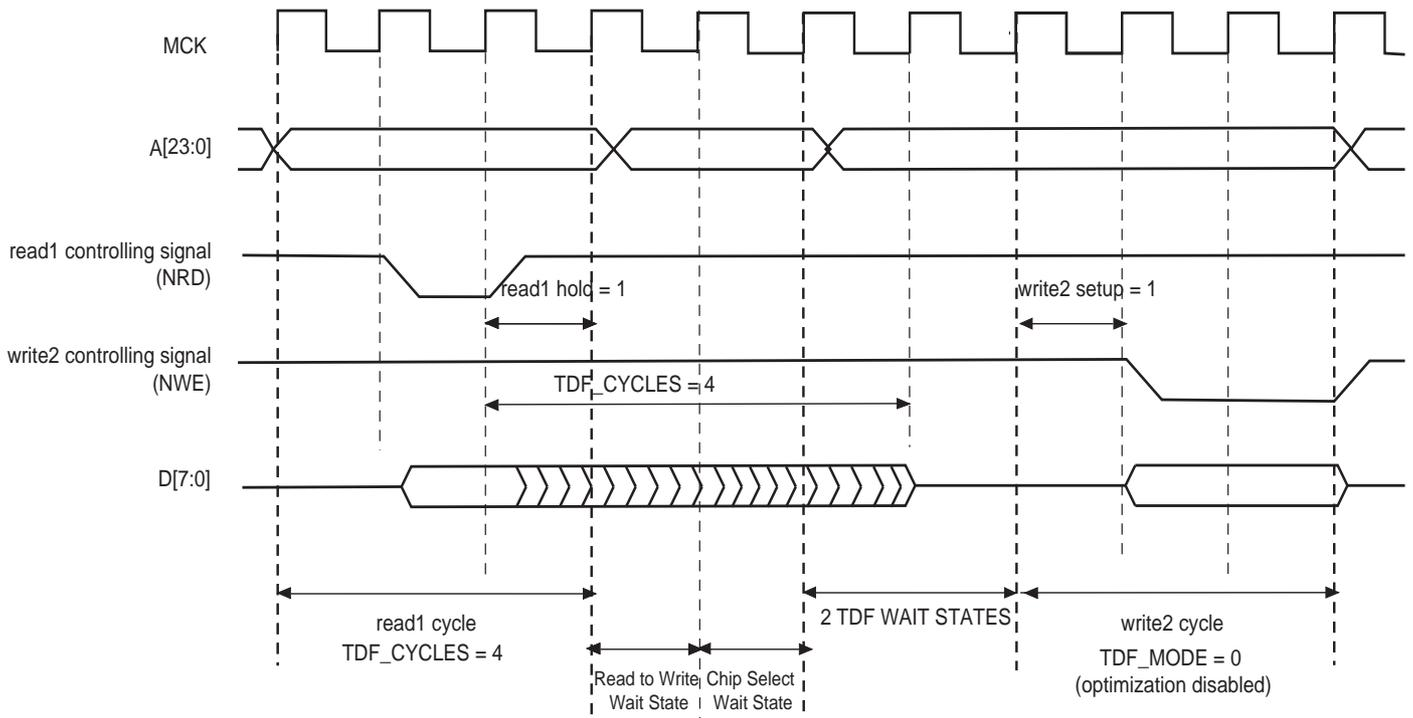
Figure 26-22. TDF Mode = 0: TDF wait states between read and write accesses on the same chip select
