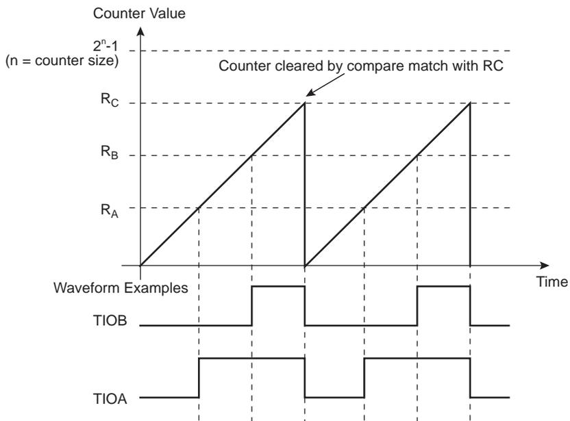
**Figure 37-10. WAVSEL = 10 with Trigger**
