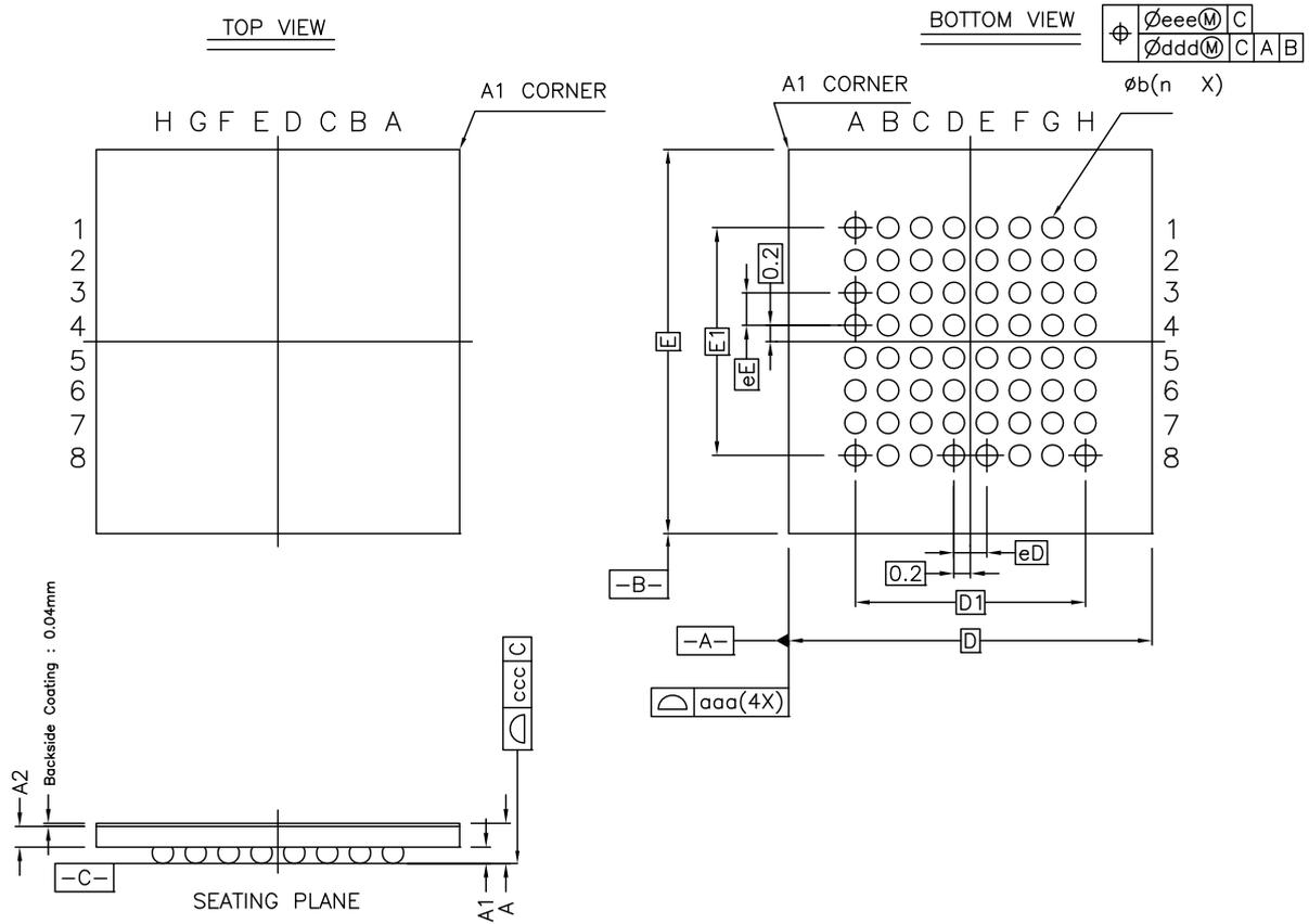
**Figure 45-7. 64-ball WLCSP Package Mechanical Drawing (SAM4S16/SAM4S8/SAM4S4/SAM4S2)**
