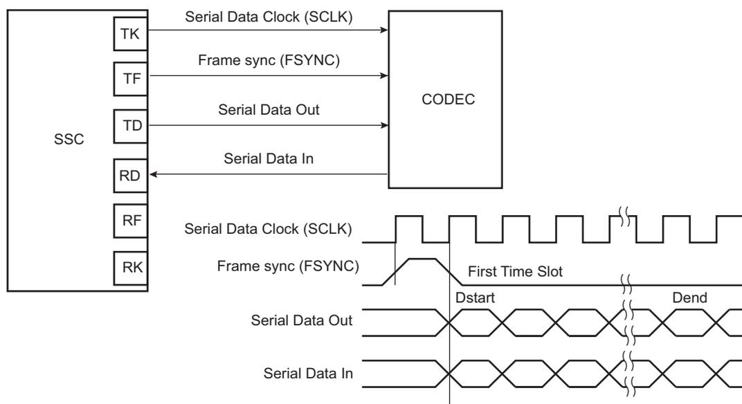
**Figure 32-5. Time Slot Application Block Diagram**
