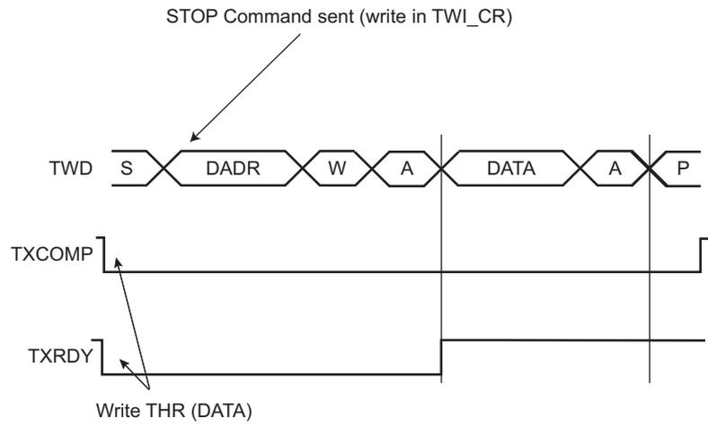
**Figure 34-6. Master Write with Multiple Data Bytes**
