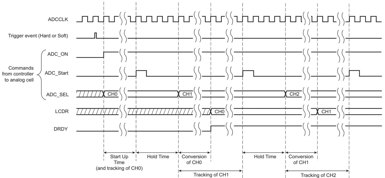
**Figure 42-3. Sequence of ADC Conversions When Tracking Time < Conversion Time**
