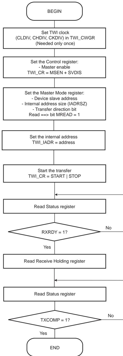
**Figure 34-19. TWI Read Operation with Multiple Data Bytes with or without Internal Address**
