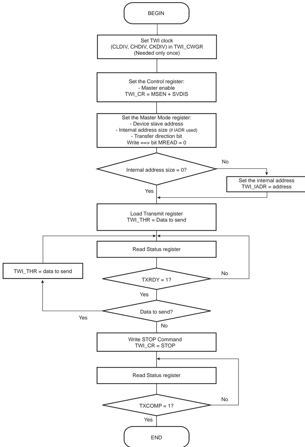
**Figure 34-17. TWI Read Operation with Single Data Byte without Internal Address**
