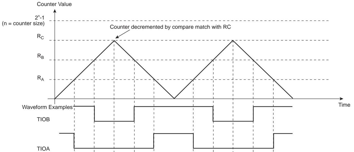
**Figure 37-14. WAVSEL = 11 with Trigger**
