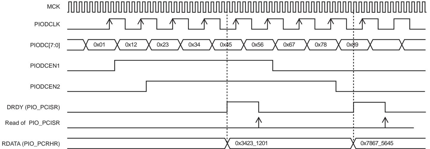
**Figure 31-11. Parallel Capture Mode Waveforms (DSIZE = 2, ALWAYS = 0, HALFS = 1, FRSTS = 0)**
