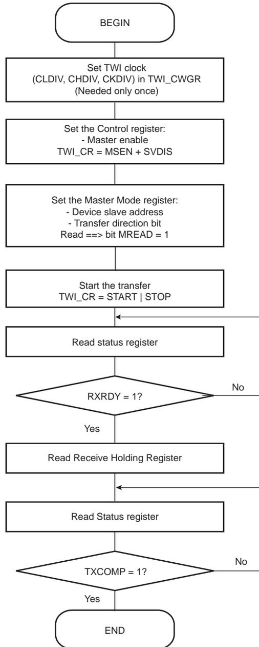
Figure 34-18. TWI Read Operation with Single Data Byte and Internal Address
