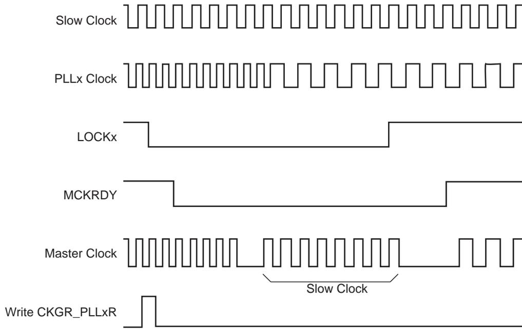
**Figure 29-9. Programmable Clock Output Programming**
