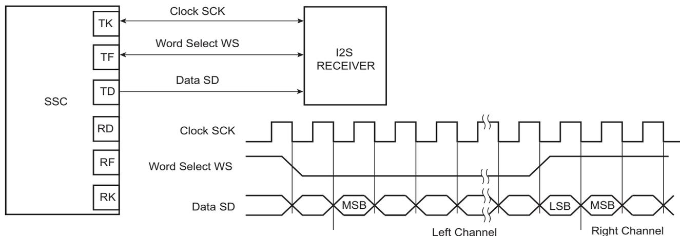
**Figure 32-4. Codec Application Block Diagram**
