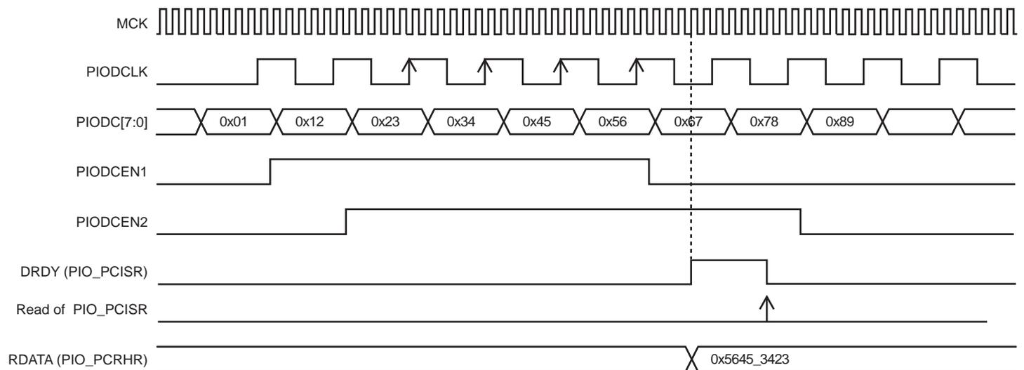
**Figure 31-10. Parallel Capture Mode Waveforms (DSIZE = 2, ALWAYS = 1, HALFS = 0)**
