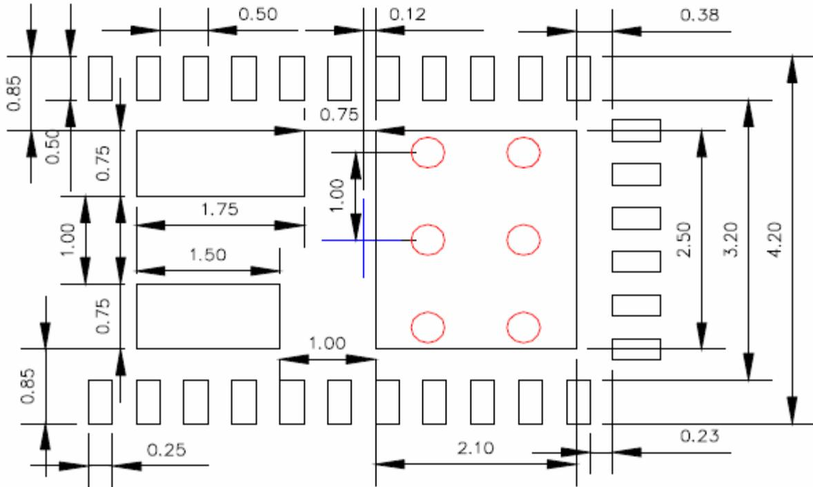
**Red circle** indicates Thermal Via. Size should be .300-.350 mm in diameter and it should be connected to GND plane for maximum thermal performance.
