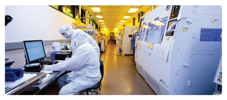
Merit Sensor owns and operates a MEMS wafer fab, which enables the production of customized piezoresistive pressure sensors.
