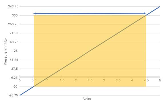
Compound sensor (measuring both vacuum and gage; both sides of zero)
