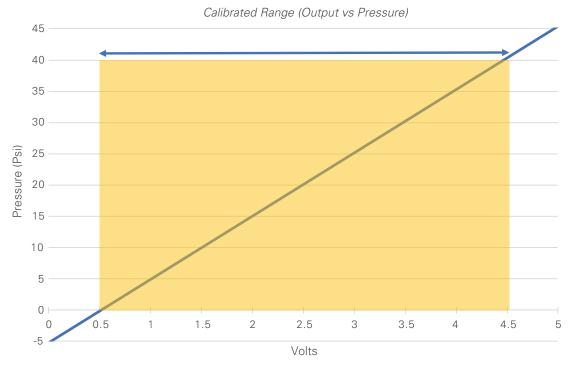
Gage sensor Output = 0.5V to 4.5V Pressure = 0 to +40psi
