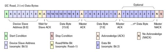
A read command will return the data from the output register. It will not interrupt the normal processing of the ASIC. Three bytes of data should be read... the first byte is the original command (0x2E), the next two bytes are the pressure output in counts.
