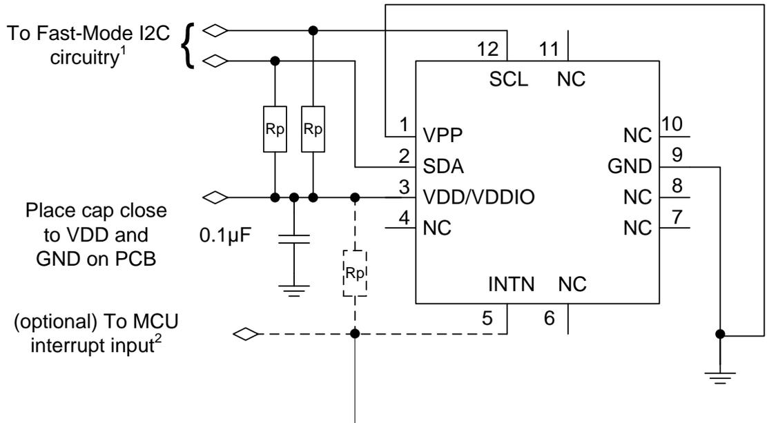
NOTE<sup>1</sup>: Rp are typically 4.7kΩ pullup resistors to VDD/VDDIO, per I2C specification. When pin VDD/VDDIO is powered down, SDA and SCL will be driven low by internal ESD diodes.
