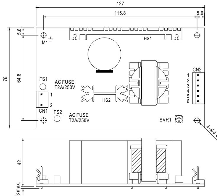
AC Input Connector (CN1) : Molex 5277-02 or equivalent
