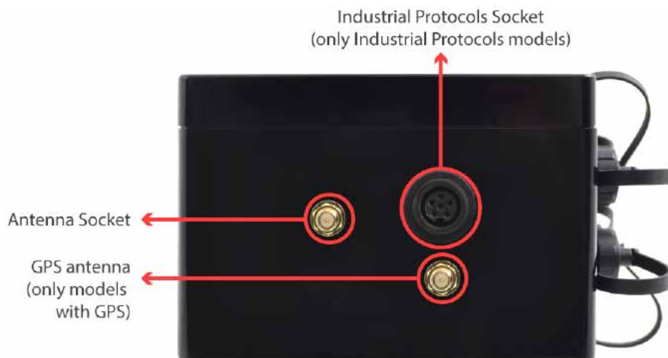
Figure: Antenna side of the enclosure
