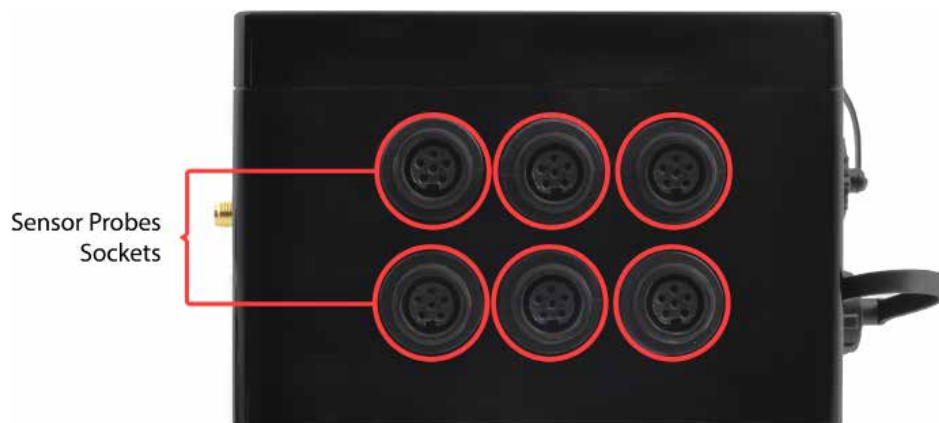
Figure: Sensor side of the enclosure
