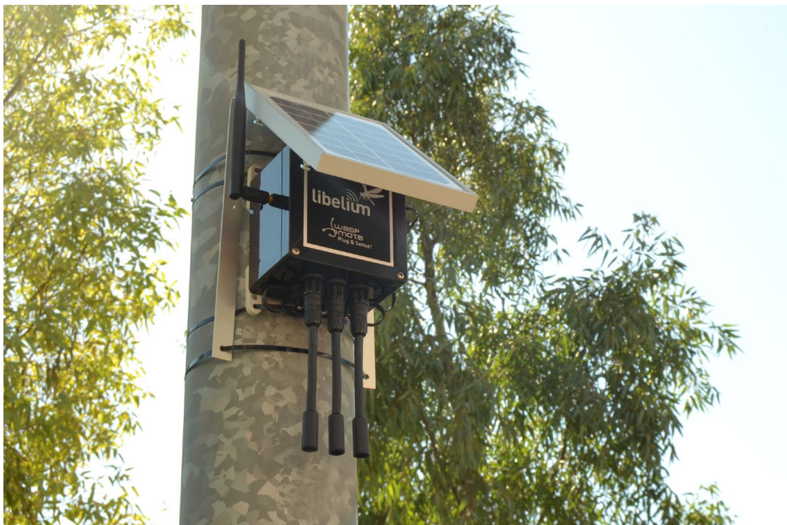
Figure : Wasp mote Plug & Sense! powered by an external solar panel
