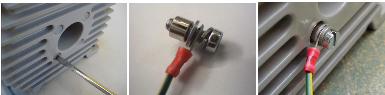
Figure 29: Attachment of a protective earth wire to the backside of the motor (Screw dimensions: M5 x 15 mm, spacer dimensions: OD = 9mm, ID = 6 mm, Length = 6 mm)
