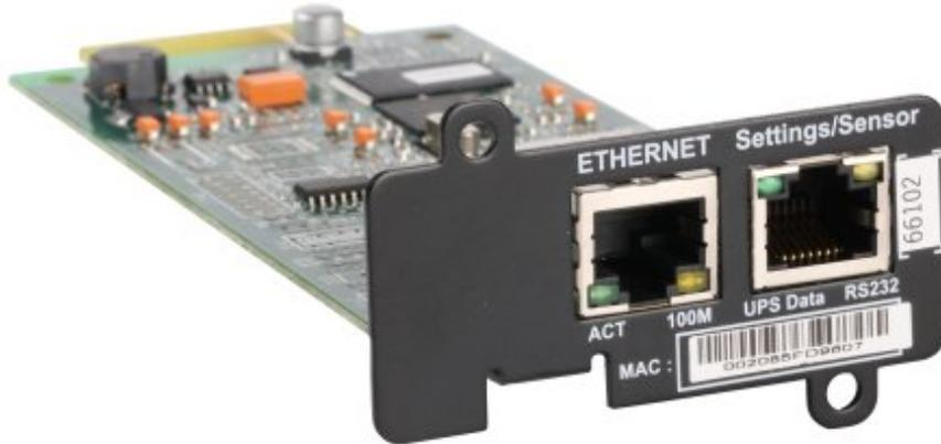
Figure 6. IBM LCD UPS Network Management Card (NMC)
