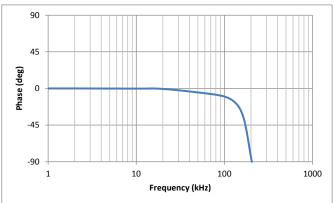
Figure 5: Typical frequency response, small signal bandwidth
