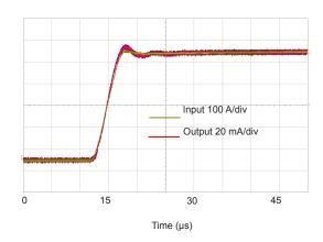
Figure 2: Typical step response (0 to 500 A, 100 A/ $\mu$ s  $R_{\rm M}$  = 1  $\Omega$ )
