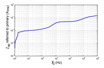
Figure 4: Typical total output current noise with  $R_{\rm M}$  = 100  $\Omega$  (primary referred, rms)
