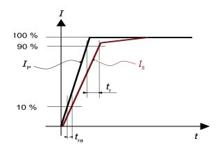
Figure 6: Response time  $t_r$  and reaction time  $t_{ra}$
