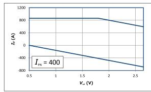
Upper limit:  $I_p = 864 \ (V_{ref} = 0.5 ... 1.8 \ V)$ Upper limit:  $I_p = -320 \times V_{ref} + 1440 \ (V_{ref} = 1.8 ... 2.65 \ V)$
