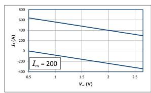
Upper limit:  $I_p = -160 \times V_{ref} + 720 (V_{ref} = 0.5 ... 2.65 V)$
