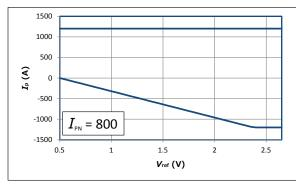
Upper limit:  $I_p = 1200 \ (V_{ref} = 0.5 ... 2.0 \ V)$ Upper limit:  $I_p = -640 \times V_{ref} + 2880 \ (V_{ref} = 2.625 ... 2.65 \ V)$
