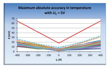
Curves in red line represent the tolerance Curves in dotted blue line represent average + 3 sigma.
