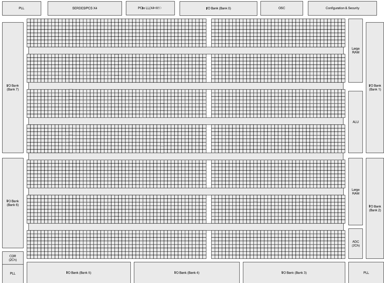
Figure 2.1. Simplified Block Diagram, LFCPNX-50 Device (Top Level)
