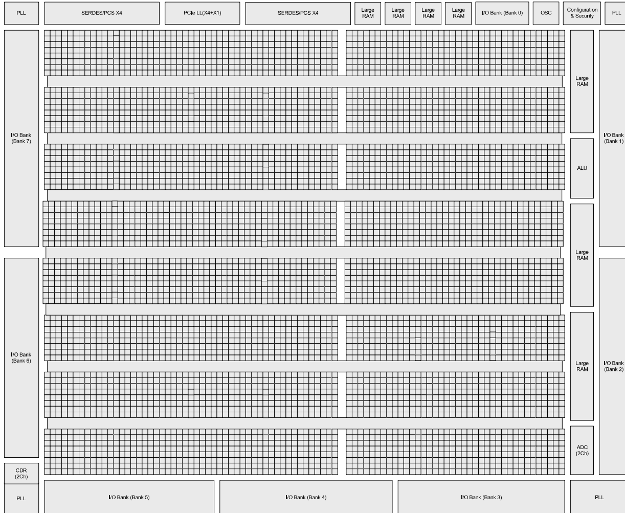
Figure 2.2. Simplified Block Diagram, LFCPNX-100 Device (Top Level)
