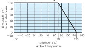
在环境温度70℃以上使用时,应按照上图负荷减轻特性曲线,减小额定功率。 For resistors operated at an ambient temperature of 70°C or above, a power rating shall be derated in accordance with the above derating curve.
