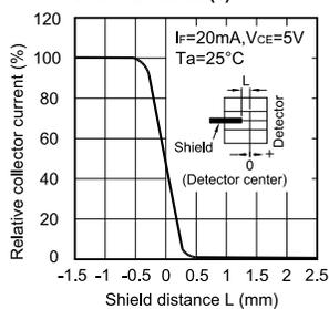
Fig. 7 Relative Collector Current vs. Shield Distance (2)
