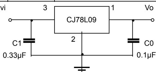
Note 1:Bypass capacitors are recommended for optimum stability and transient response and should be located as close as possible to the regulators
