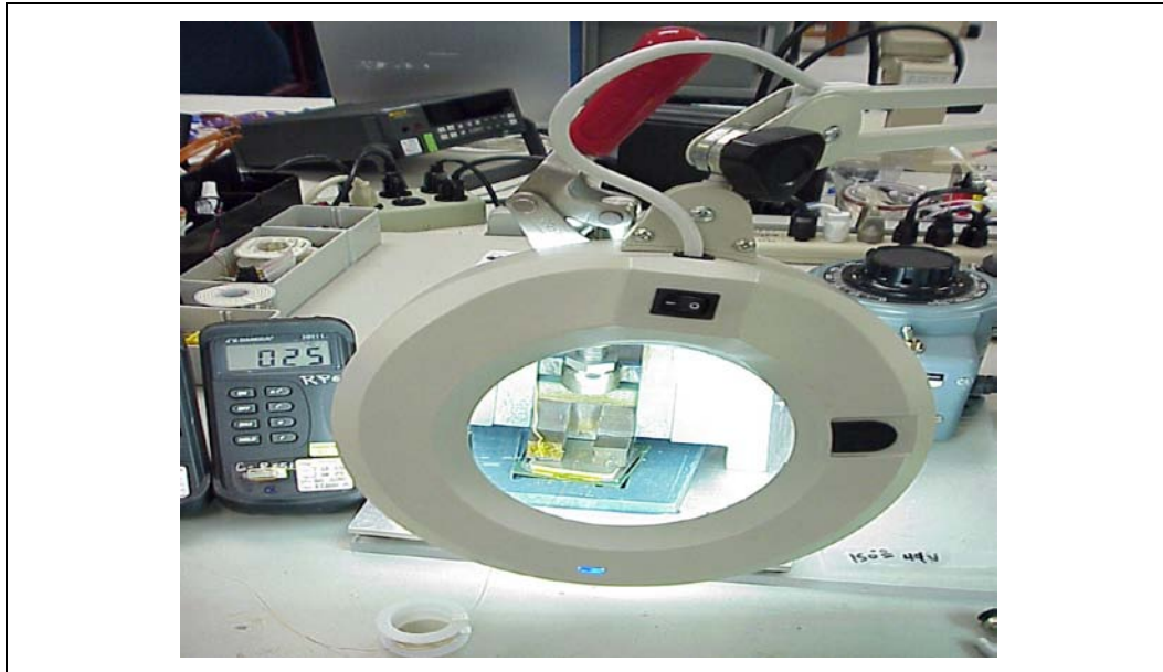
Figure 7-29. Moving Solder back onto Thermocouple Bead
