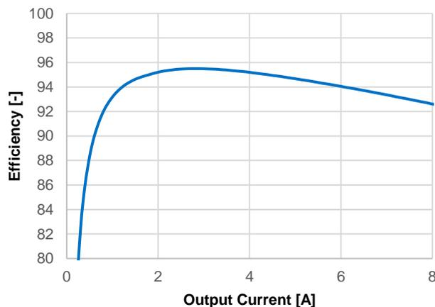
**Figure 6: Efficiency  $V_{IN} = 5.5V$ ,  $V_{OUT} = 3.3V$**
