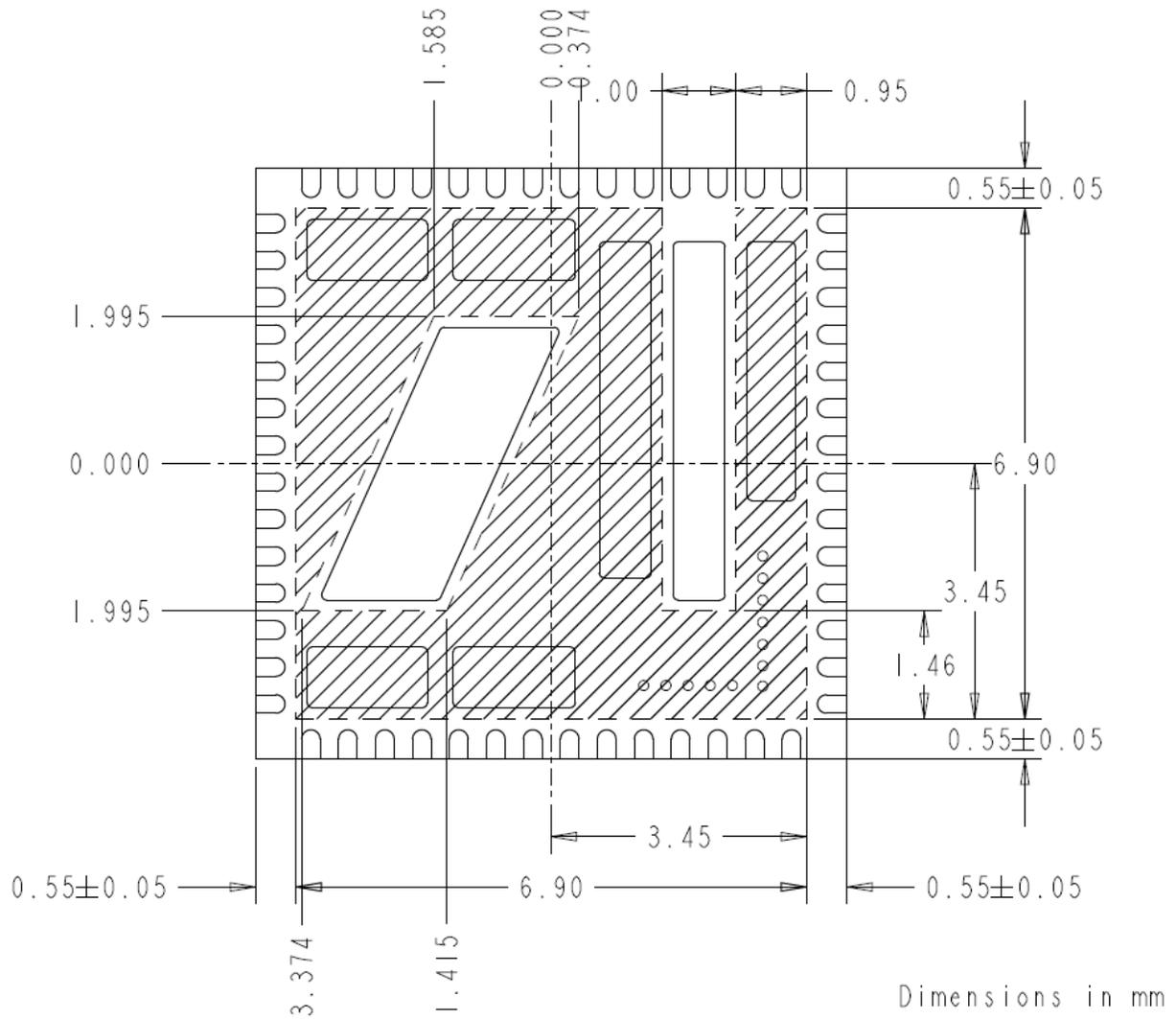
**Figure 13: EN6382QI Package – PCB Footprint Keepout (Bottom view)**
