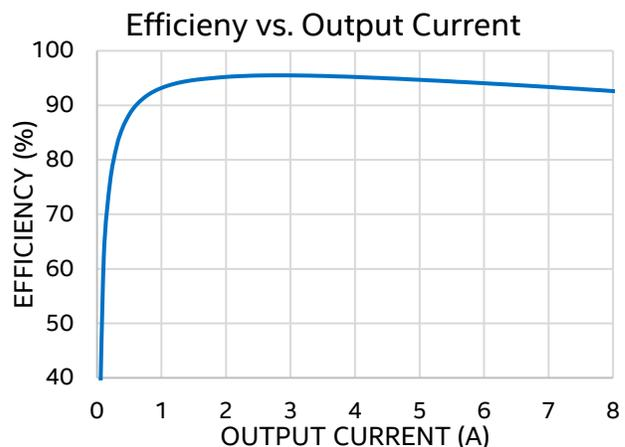
Figure 2: Efficiency at VIN = 5V, VOUT = 3.3V
