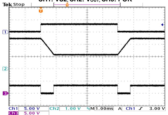
**Power Up/Down at No Load ( $V_{IN} = 5\text{ V}$ ,  $V_{OUT} = 1.2\text{ V}$ )**
