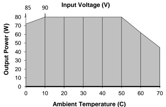
Derating requirements - Derate from 100% load at 50°C to 50% load at 70°C.
