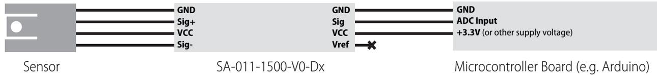
**Differential operation:** The amplifier outputs «Sig» and «Vref» can be connected to a differential analog input. This is the recommended configuration for the **-V10-** variants. The output signal against Vref will be between 0 and 10 V (**-V10-D1**) or between  $-5$  and  $+5$  V (**-V10-D2**), respectively.
