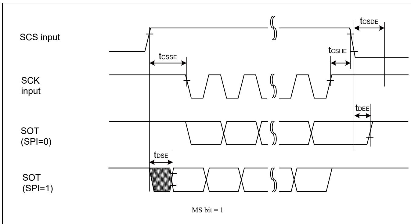
**When using synchronous serial chip select (SCINV = 1, CSLVL=0)**
