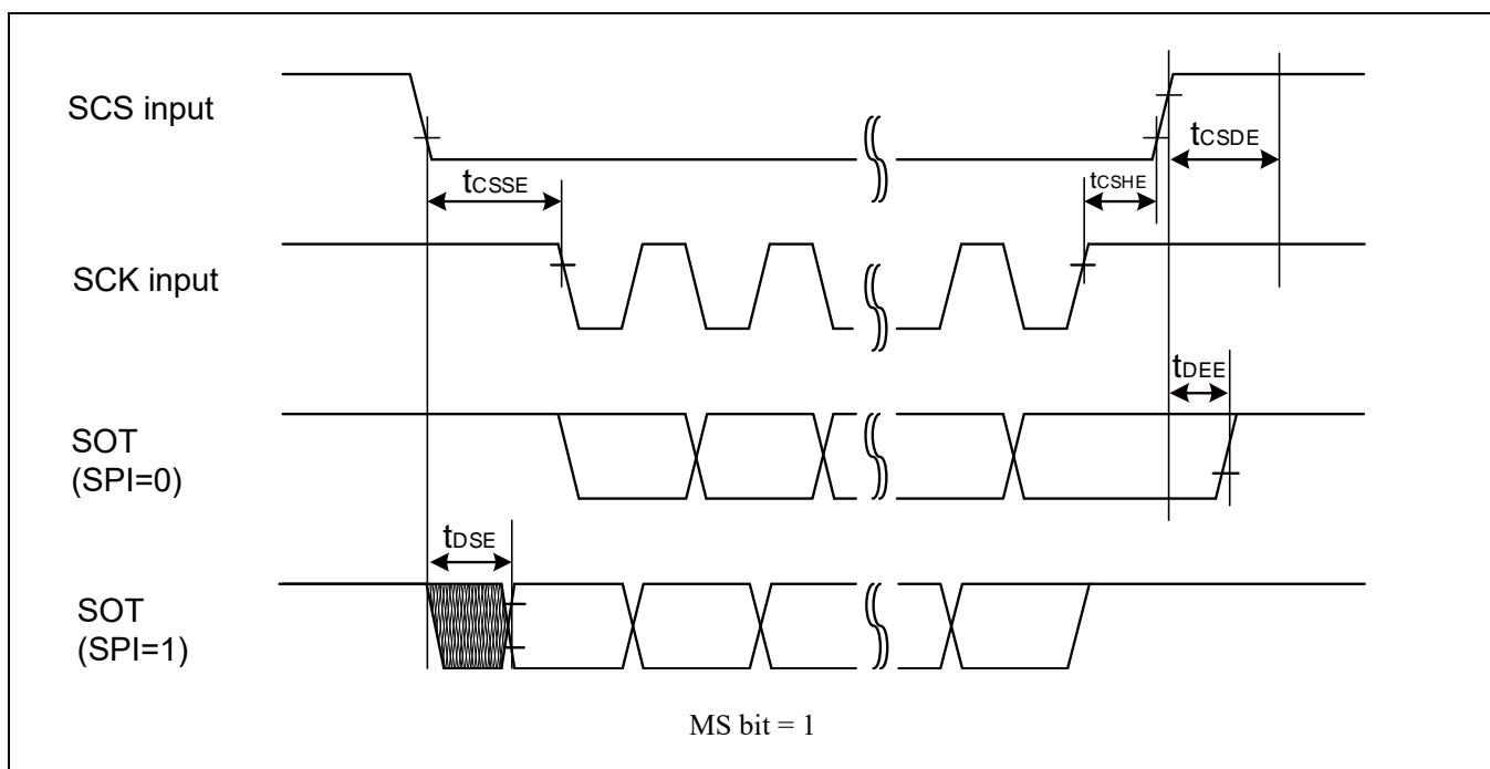
**When using synchronous serial chip select (SCINV = 1, CSLVL=1)**
