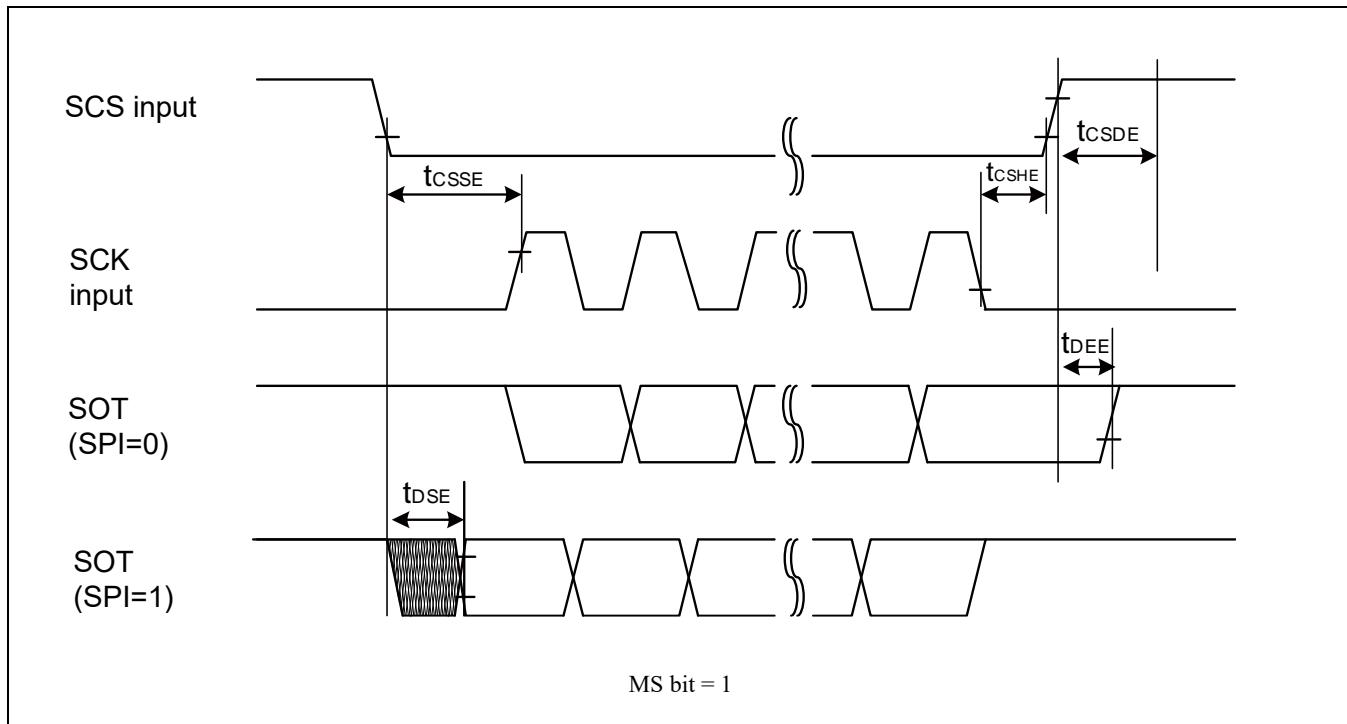
**When using synchronous serial chip select (SCINV = 0, CSLVL=0)**
