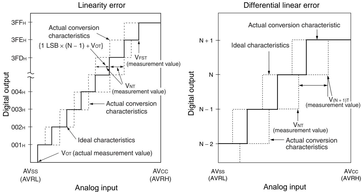
$$\text{Linear error in digital output } N = \frac{V_{NT} - \{1 \text{ LSB} \times (N - 1) + V_{OT}\}}{1 \text{ LSB}} \quad [\text{LSB}]$$
