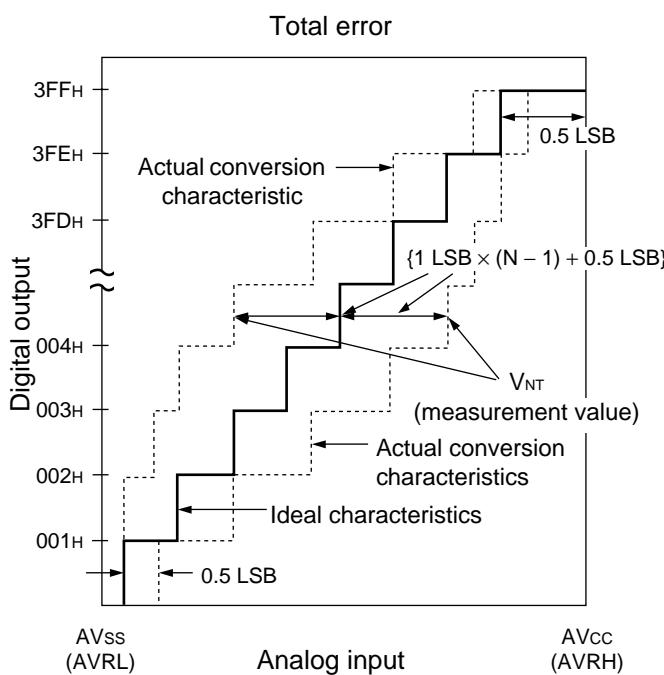
$$\text{Total error of digital output } N = \frac{V_{NT} - \{1 \text{ LSB} \times (N - 1) + 0.5 \text{ LSB}\}}{1 \text{ LSB}} \text{ [LSB]}$$
