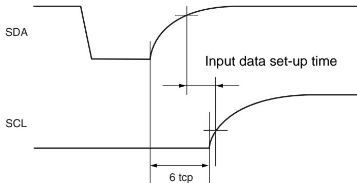
Note : The rating of the input data set-up time in the device connected to the bus cannot be satisfied depending on the load capacitance or pull-up resistor.
