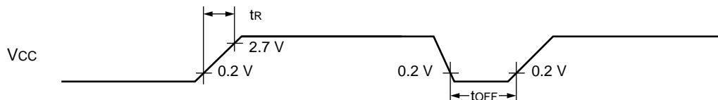
Note : Sudden change of power supply voltage may activate the power-on reset function. When changing power supply voltages during operation, raise the power smoothly by suppressing variation of voltages as shown below.
