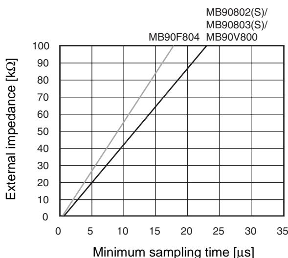
(External impedance = 0 k $\Omega$  to 20 k $\Omega$ )
