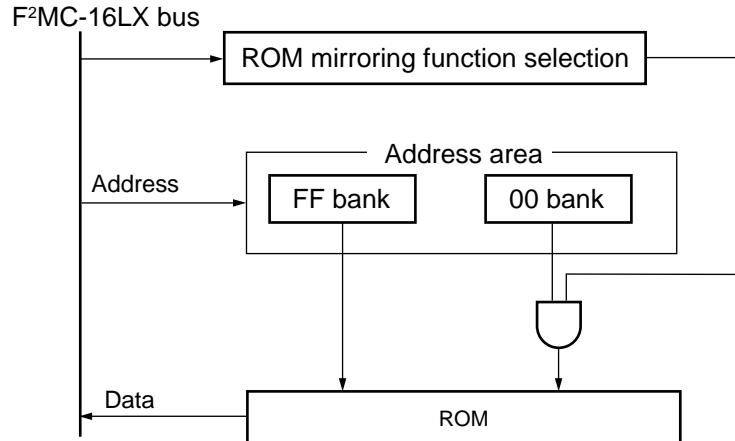
Note : Do not access to ROM mirroring function selection register in the middle of the operation of the address 008000<sub>H</sub> to 00FFFF<sub>H</sub>.
