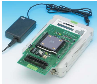
Main unit and adaptor board of the 16LX high-speed emulator
