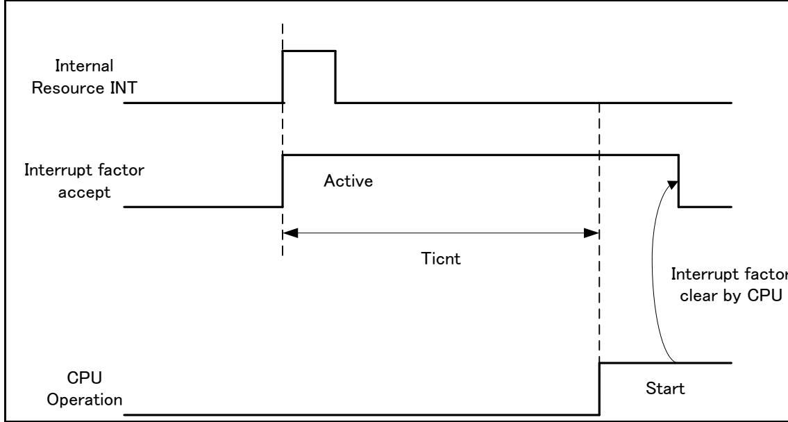
\*: Depending on the standby mode, interrupt from the internal resource is not included in the recovery cause.
