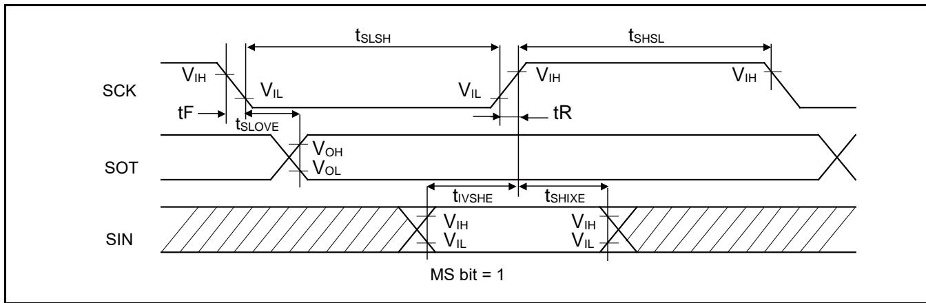
**High-Speed Synchronous Serial (SPI = 0, SCINV = 1)**
