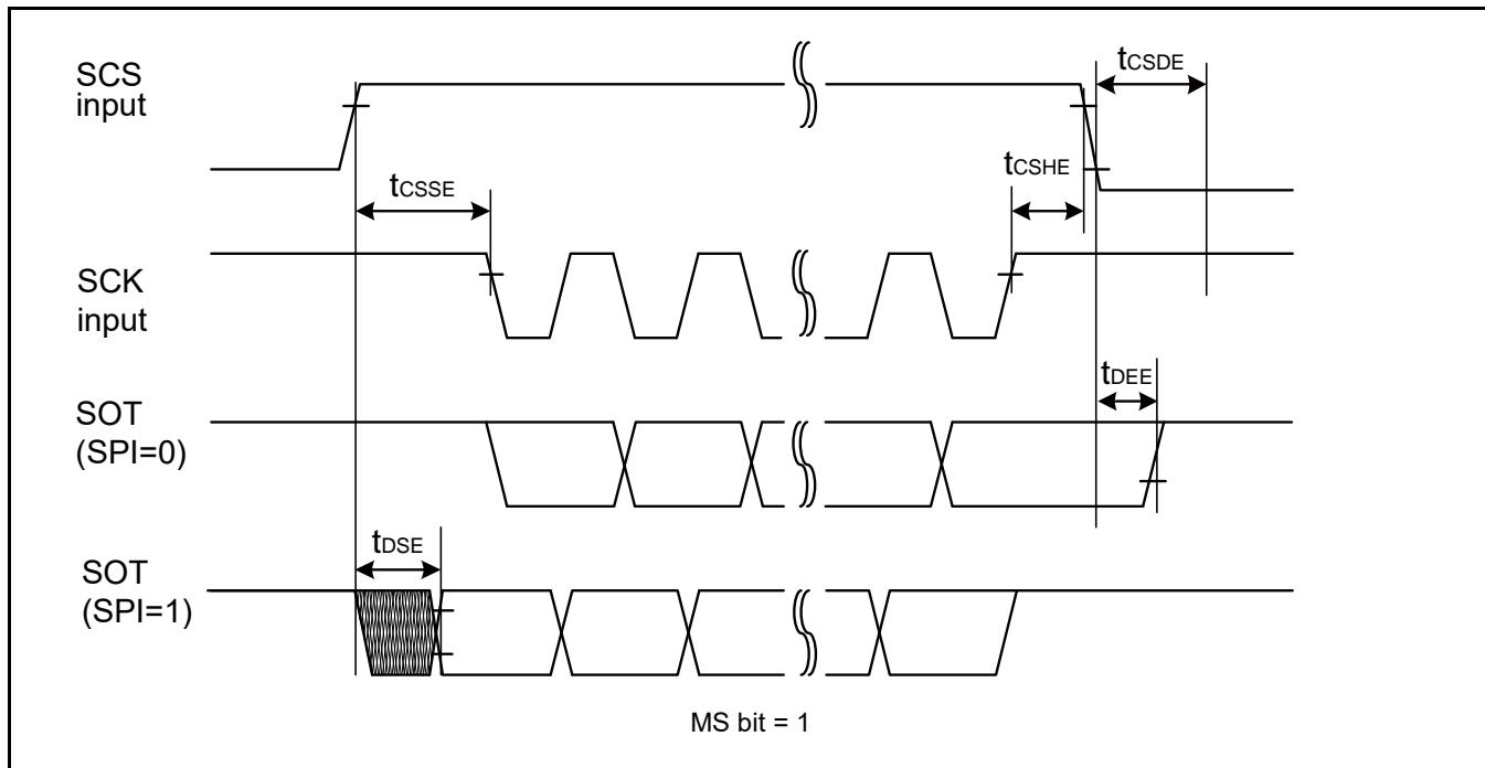
**When Using High-Speed Synchronous Serial Chip Select (SCINV = 1, CSLVL=0)**
