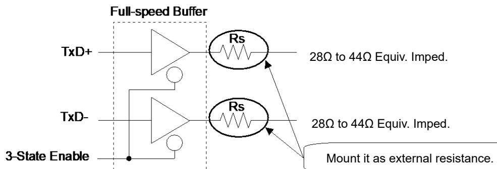
$R_s$  series resistor  $25\ \Omega$  to  $30\ \Omega$
