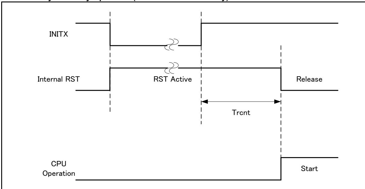
**Example of Standby Recovery Operation (when in Internal Resource Reset Recovery\*)**
