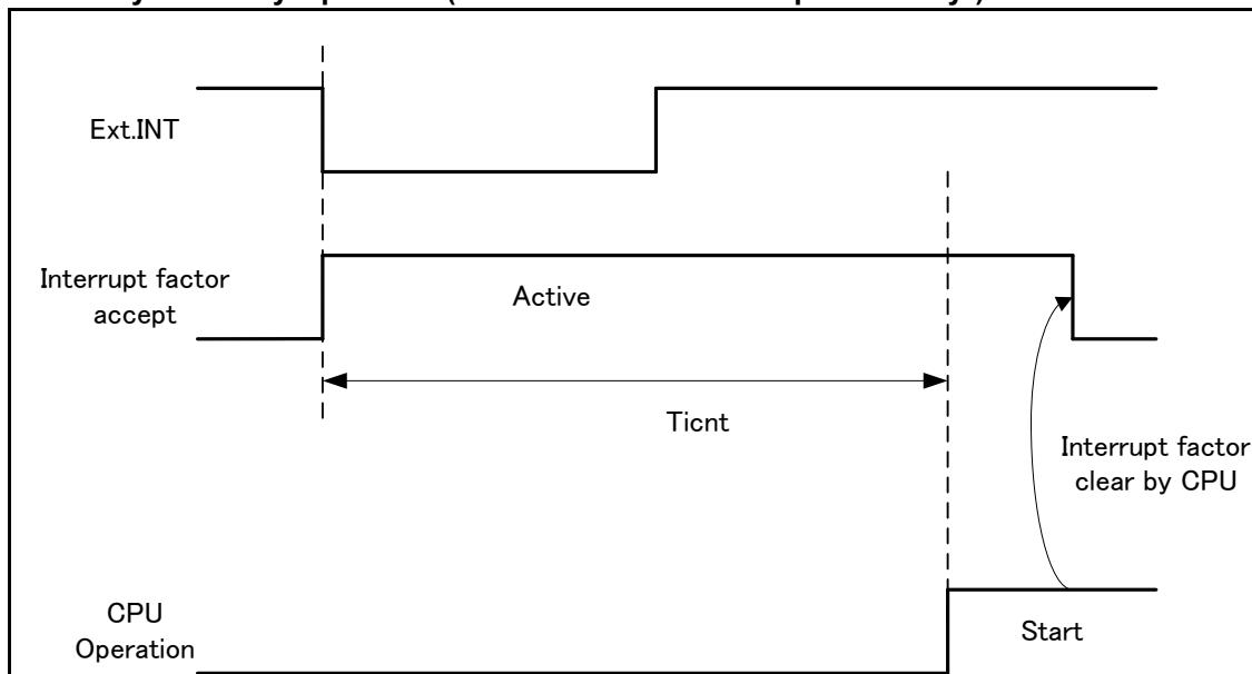
\*: External interrupt is set to detecting fall edge.
