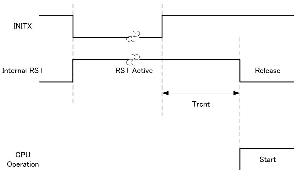
**Example of standby recovery operation (when in internal resource reset recovery\*)**
