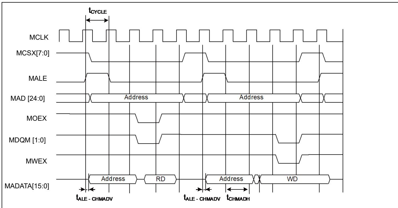
**Multiplexed Bus Access Synchronous SRAM Mode**
