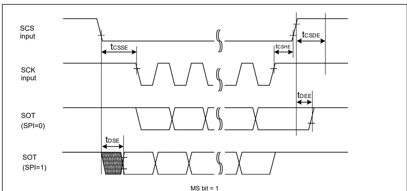
**When using synchronous serial chip select (SCINV = 1, CSLVL = 1)**
