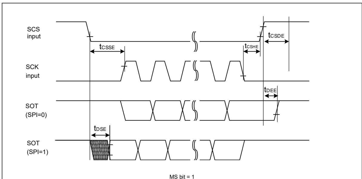
**When using synchronous serial chip select (SCINV = 0, CSLVL = 0)**
