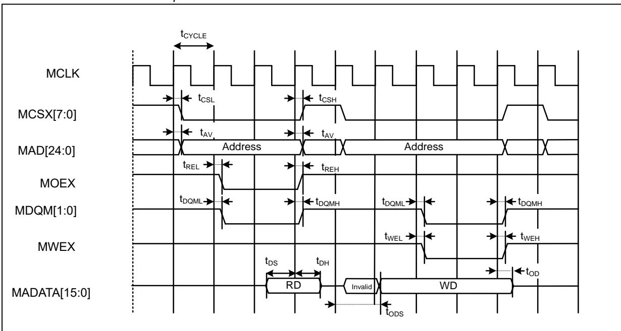
**Multiplexed Bus Access Asynchronous SRAM Mode**
