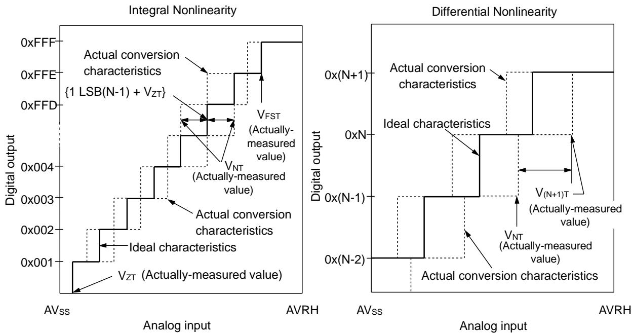
$$\text{Linearity error of digital output } N = \frac{V_{NT} - \{1\text{LSB} \times (N - 1) + V_{ZT}\}}{1\text{LSB}} \text{ [LSB]}$$
