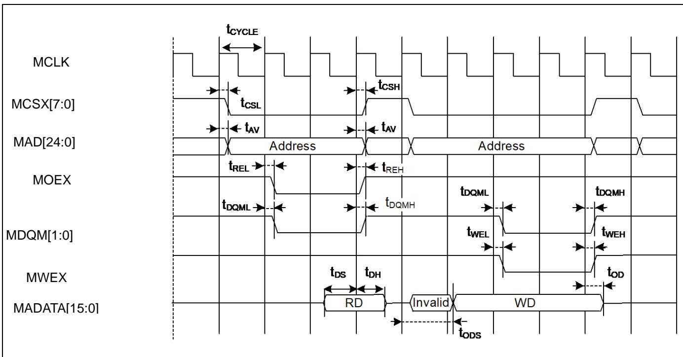
**Multiplexed Bus Access Asynchronous SRAM Mode**
