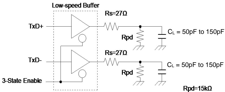
**Low-Speed Load (Downstream Port Load) - Reference 2**
