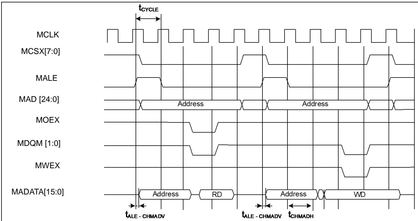
**Multiplexed Bus Access Synchronous SRAM Mode**
