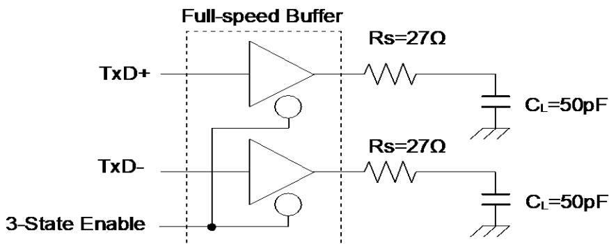
6: USB Full-speed connection is performed via twist pair cable shield with  $90\Omega \pm 15\%$  characteristic impedance (Differential Mode). USB standard defines that output impedance of USB driver must be in range from  $28\Omega$  to  $44\Omega$ . So, discrete series resistor ( $Rs$ ) addition is defined in order to satisfy the above definition and keep balance.
