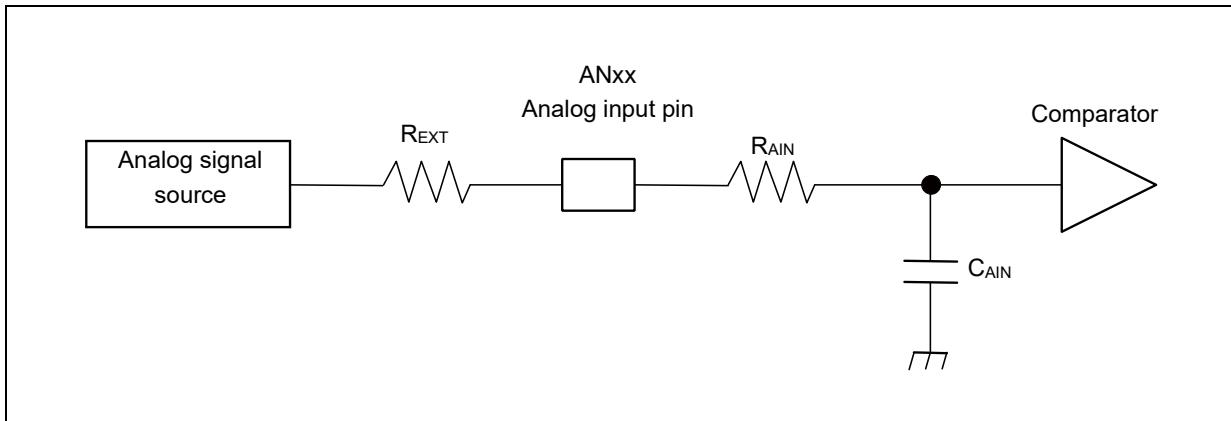
(Equation 1)  $t_s \geq (R_{AIN} + R_{EXT}) \times C_{AIN} \times 9$
