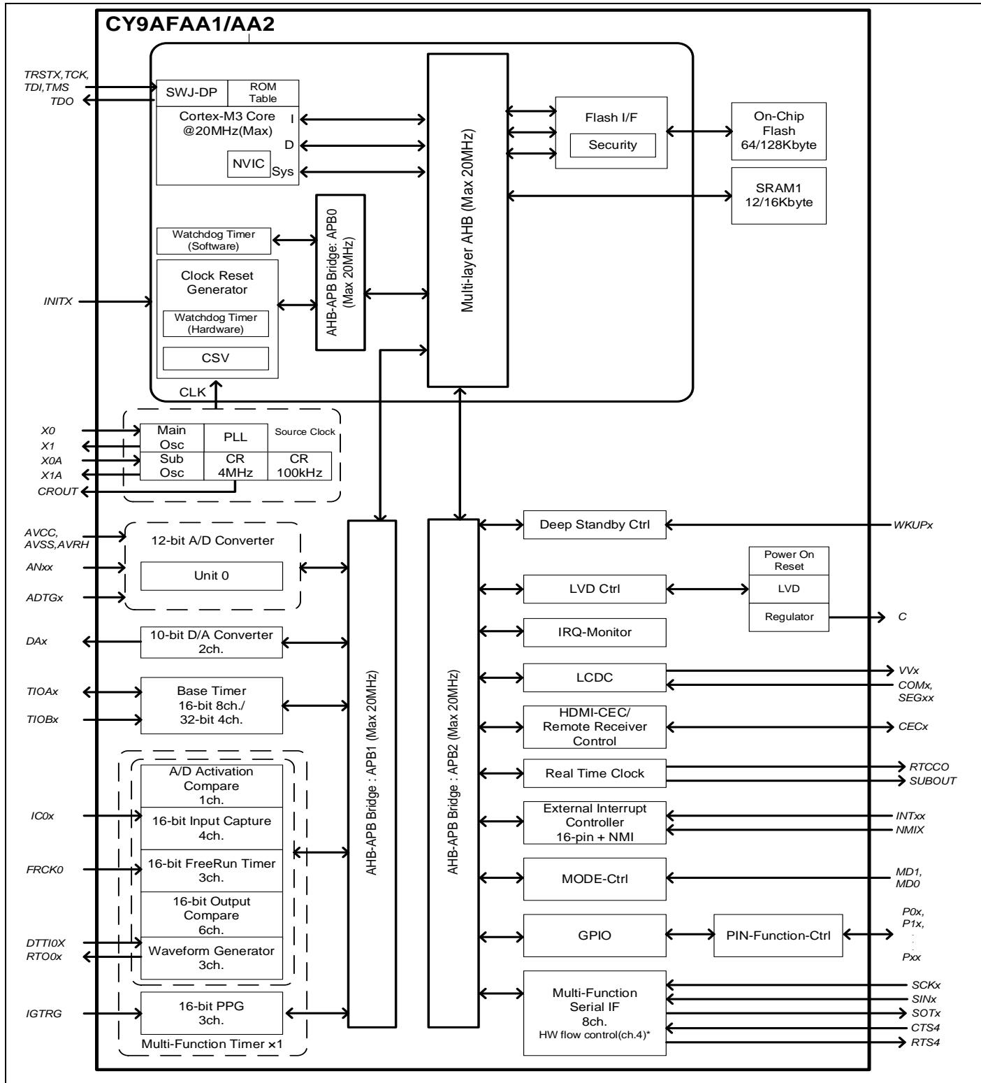
\*: For the CY9AFAA1L and CY9AFAA2L, Multi-function Serial Interface does not support hardware flow control in these products.
