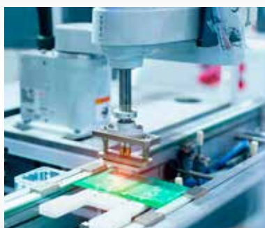
Positioning PCB conveyor lines
