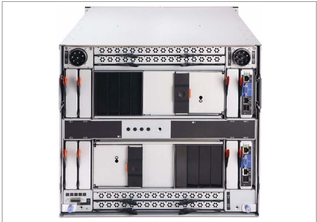
Figure 1-7 BladeCenter H rear view
