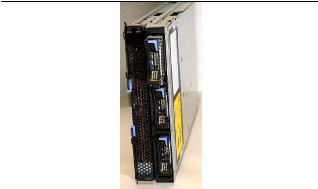
Figure 3-60 HS21 8853 with the Storage and I/O (SIO) Expansion Unit attached
