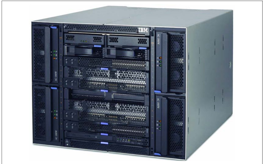
Figure 1-9 BladeCenter T front view
