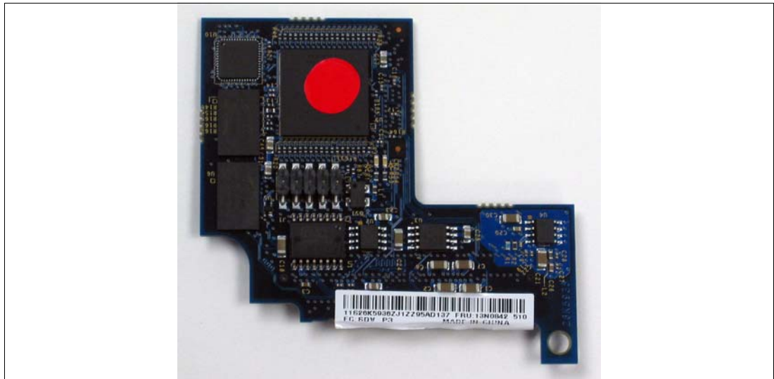
Figure 3-53 Concurrent KVM Feature Card
