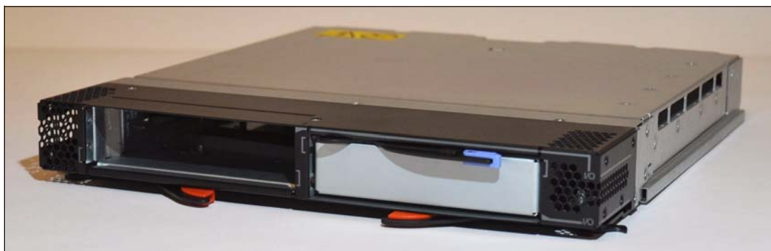
Figure 2-38 Multi-switch Interconnect Module for BladeCenter HT (without interposers)
