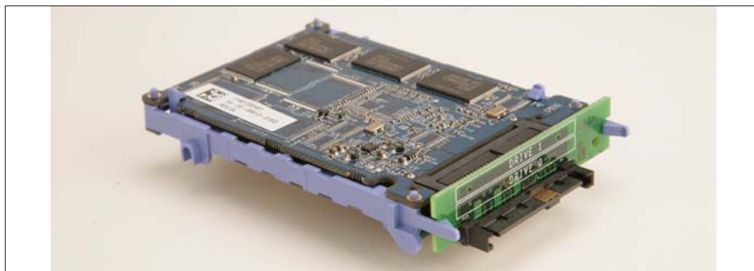
Figure 3-39 A Dual 15.8 GB Solid State Drive option
