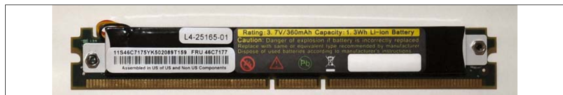
Figure 3-23 The Battery Backup unit for the ServeRAID-MR10ie (CIOv) Controller
