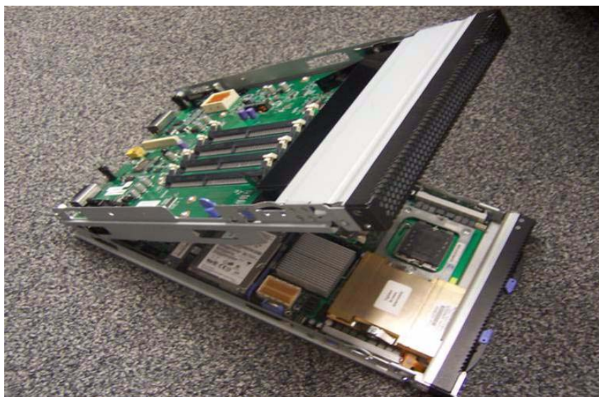
Figure 3-57 Memory and I/O (MIO) Expansion Unit attached to the HS21
