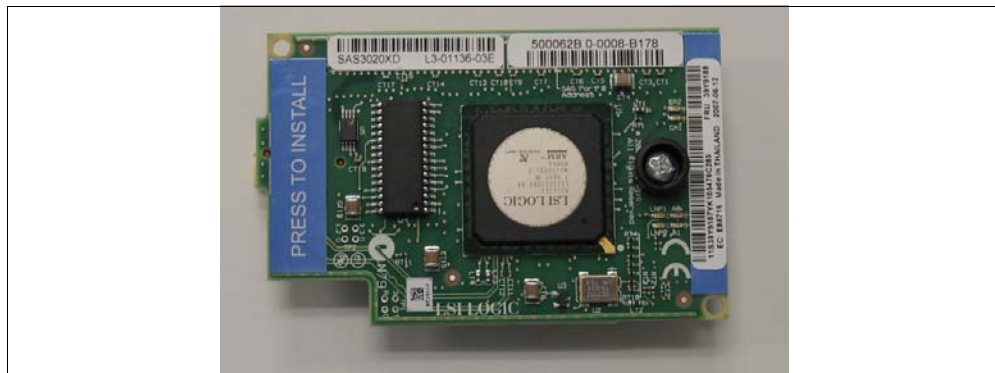
Figure 3-20 SAS Expansion Card (CFFv)
