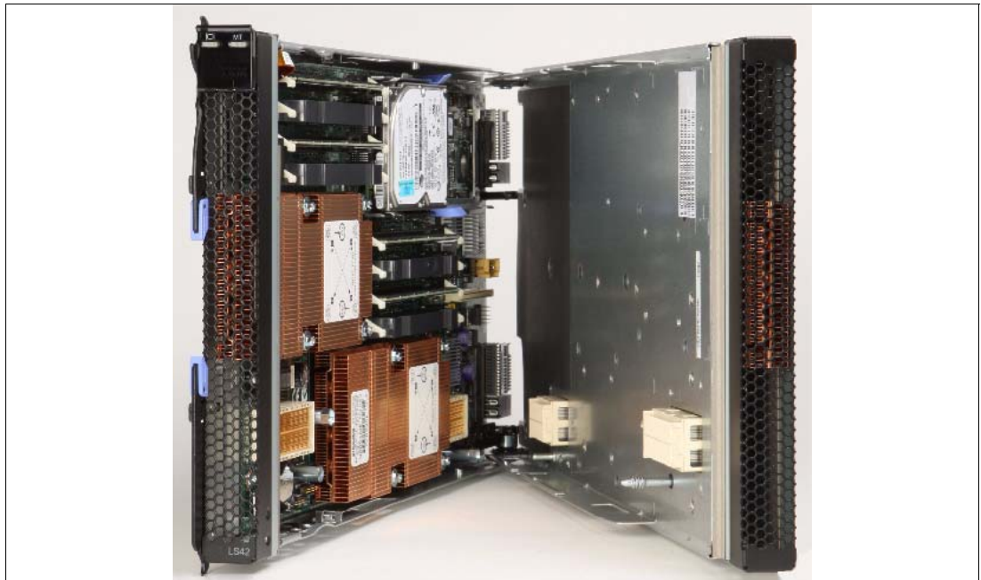
Figure 1-28 IBM BladeCenter LS42 and MPE unit
