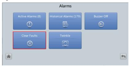
Figure 5-16 Clearing the alarm
