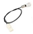
500 Series surface temperature probe, NTC, 10,000 Ohm,  $\pm 5.0\%$ tolerance, 25 °C [77 °F] accuracy, nickel-plated copper, ring tongue (#10), lead wires/AMP 172157-1, 22 gauge Teflon insulation, 102 mm [4 in]
