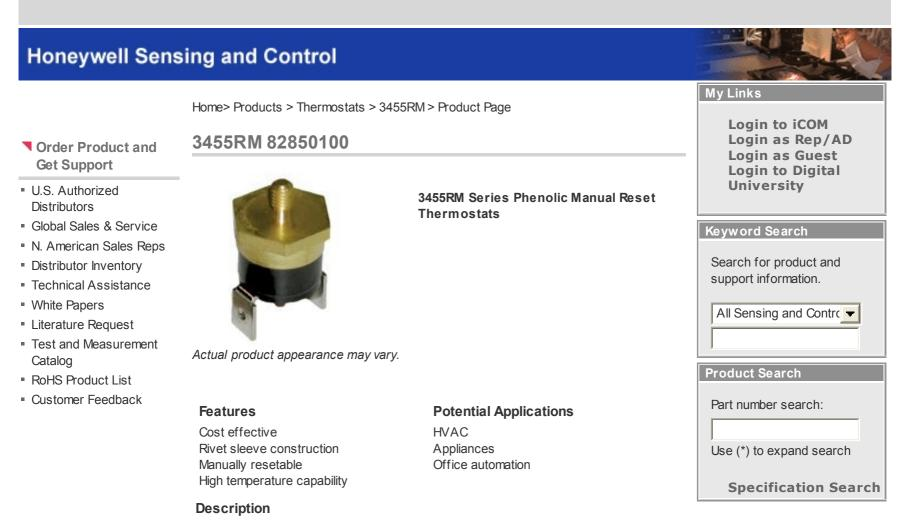
The 3455RM Series consists of a temperature-sensitive bimetal disc, electrically isolated from the switch, which actuates the normally closed contacts. The contacts open when the surface or ambient temperatures increase to the operating snap point of the calibrated disc. The circuit will stay open above room ambient temperature until the manual reset button is pressed. Response to temperature changes is extremely rapid due to the inherently low mass of the disc and the small size of the product.
